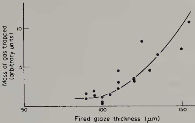
Fig. 12.2. Relationship between glaze thickness and bubble population 30
