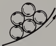
Fig. 5.1. Movement of tumbling balls in the layers adjacent to a mill lining.
