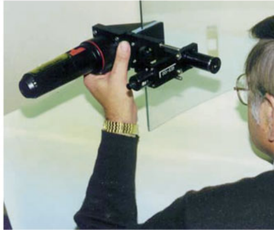
Fig. 11.9 (a) Edge stress meter principle with a Senarmont compensator. (b) Sharples edge stress meter. (Photograph courtesy of Sharples Stress Engineers Ltd, http://www.sharplestress.com/ .) (c) Strain optics Inc. edge stress meter. (Photograph courtesy of Strainoptics Inc., www.strainoptics.com .)
