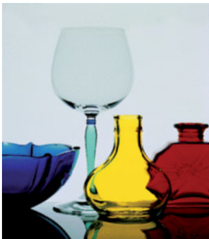
Fig. 12.24 Sol-gel film applications with decorative interest. Glassware demonstrating high quality optical appearance of crystal glass coated with dye coloured hybrid coatings. (Reprinted from Schottner, 2001, with permission from the American Chemical Society.)
