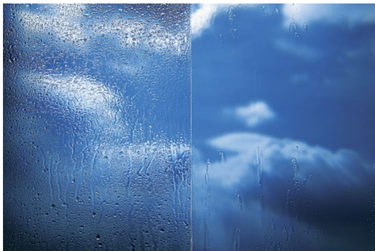
Fig. 4.4 Photograph of windows taken from indoor looking out with one ordinary window glass (left) and self cleaning glass (right). (Copyright Saint-Gobain.)
