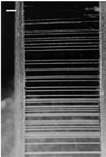
Fig. 6.38 Multiple surface cracks in a two-step ion-exchanged glass tested under four-point bending. Loading axis is perpendicular to crack direction (HF acid etching was used to widen cracks for better visibility; the white bar is 1 mm long). (From Abrams et al., 2003, with permission from Elsevier.)
