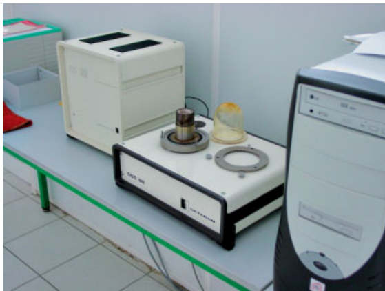
Fig. 6.12 Differential scanning calorimeter set-up.
