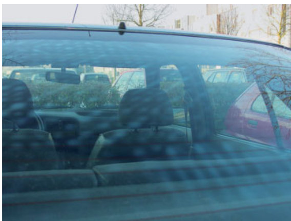
Fig. 6.27 Nozzle photoelastic signatures (due to tempering) are observed here on a backlight (they correspond to residual stress heterogeneities and are better observed at dawn; see also Chapter 11).
