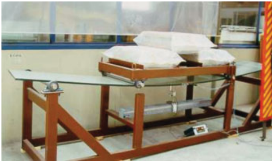
Fig. 2.11 Tempered glass beam under flexure (four-point bending). For the experiment here, the larger side is set horizontally. This set-up was used to determine the delayed elastic response (Gy, 1999; see also Chapter 6. Courtesy R. Gy, Saint Gobain Recherche.)
