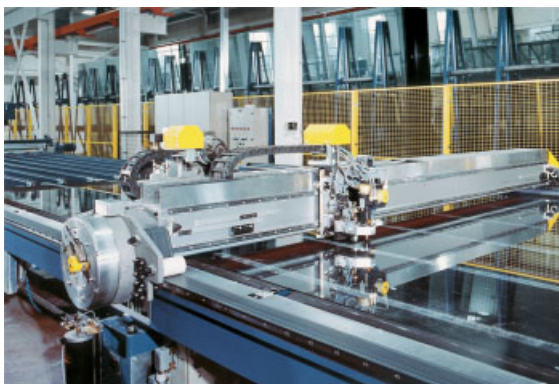
Fig. 8.28 Glass cutting machine (Bystronic Maschinen AG/ marketing brochure 2003) showing the scribing tool on a translating arm. (Courtesy of Bystronic Maschinen AG.)
