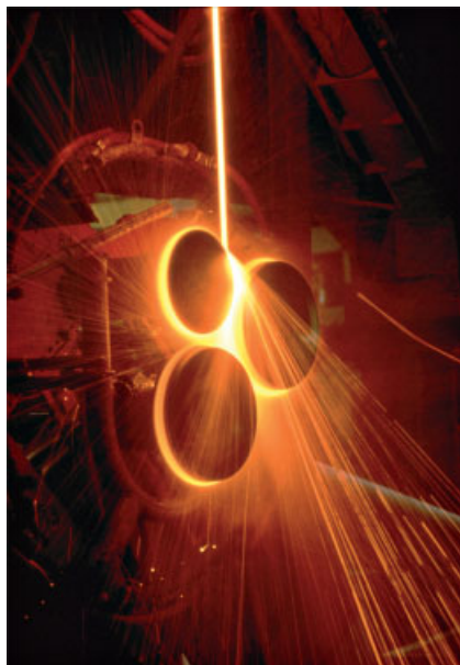
Fig. 10.16 Wool fibre wheel process. (Copyright Saint-Gobain.)
