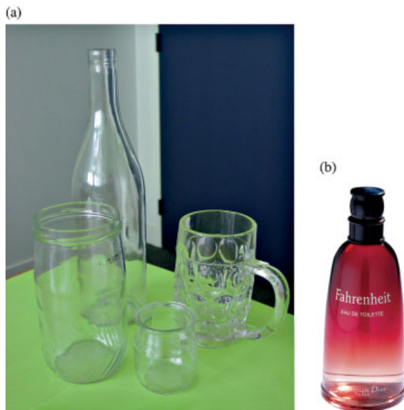
Fig. 4.6 (a) Containers and (b) fragrance flask. The fragrance bottle colour results from gold aggregates; an earlier use of this phenomenon was the ruby glass obtained by Murano glassblowers. (Copyright Saint-Gobain.)
