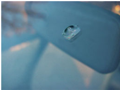
Fig. 8.8 Hertz fracture on a laminated windscreen.
