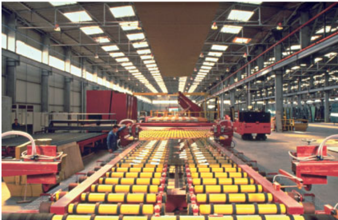
Fig. 10.3 (a) Float line at Chennai. (Copyright Saint-Gobain.) (b) Schematic representation of a float line (CVD and spray unit locations are indicated and optional). (c) Float glass line end showing transiting glass on rollers. (Copyright Saint-Gobain.)
