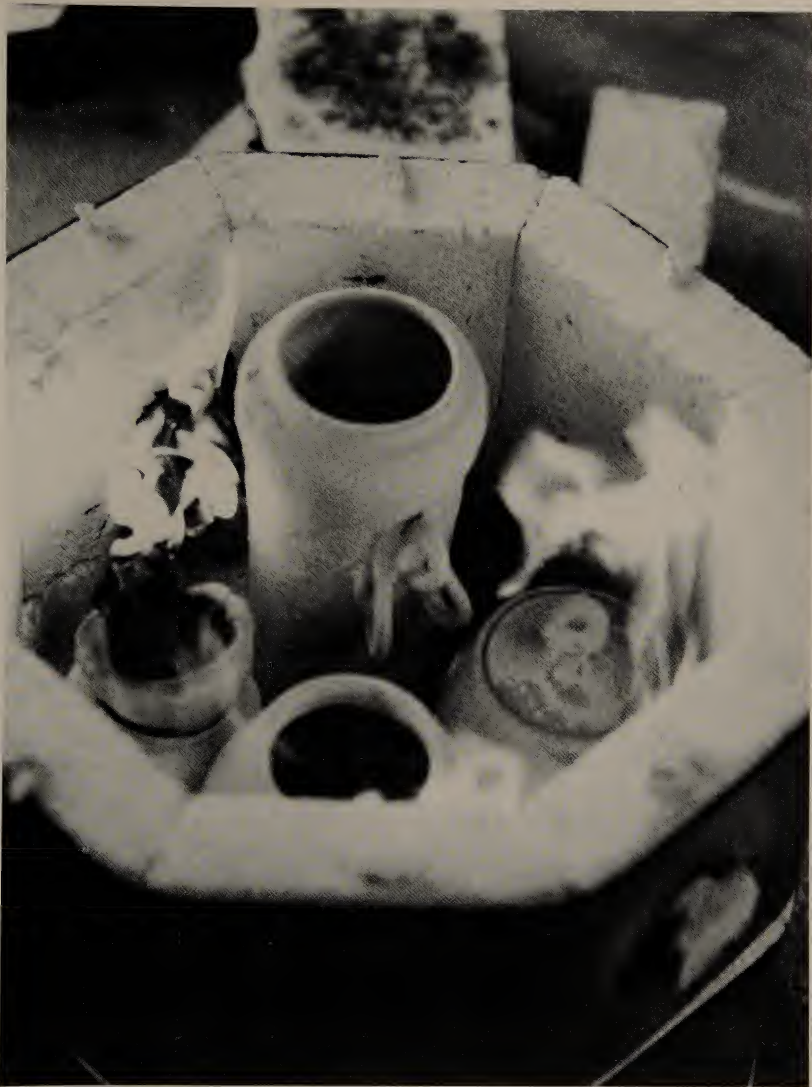
After the pieces are in position in the kiln and are not touching, the burner is slowly turned up.
