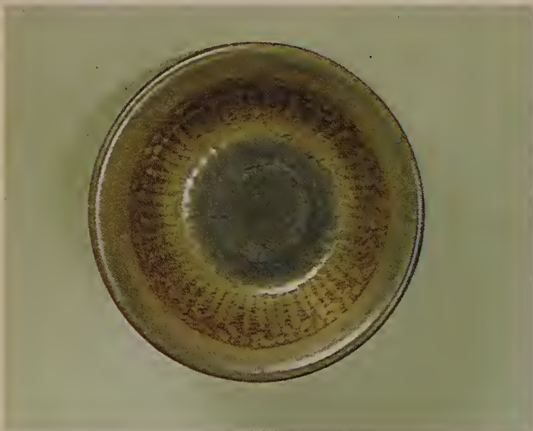
Arabian Luster Glaze R.T.-12, colored with pigment 3 and fired on schedule IV-4, results in a bright gold luster.
