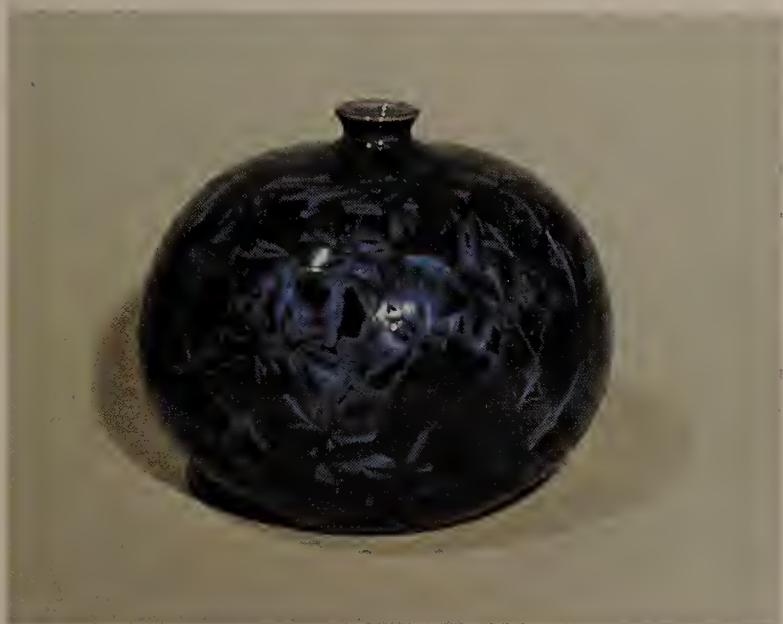
Crystalline-glazed piece illustrates Commercial Frit Glaze #1 with cobalt, manganese, and iron.
