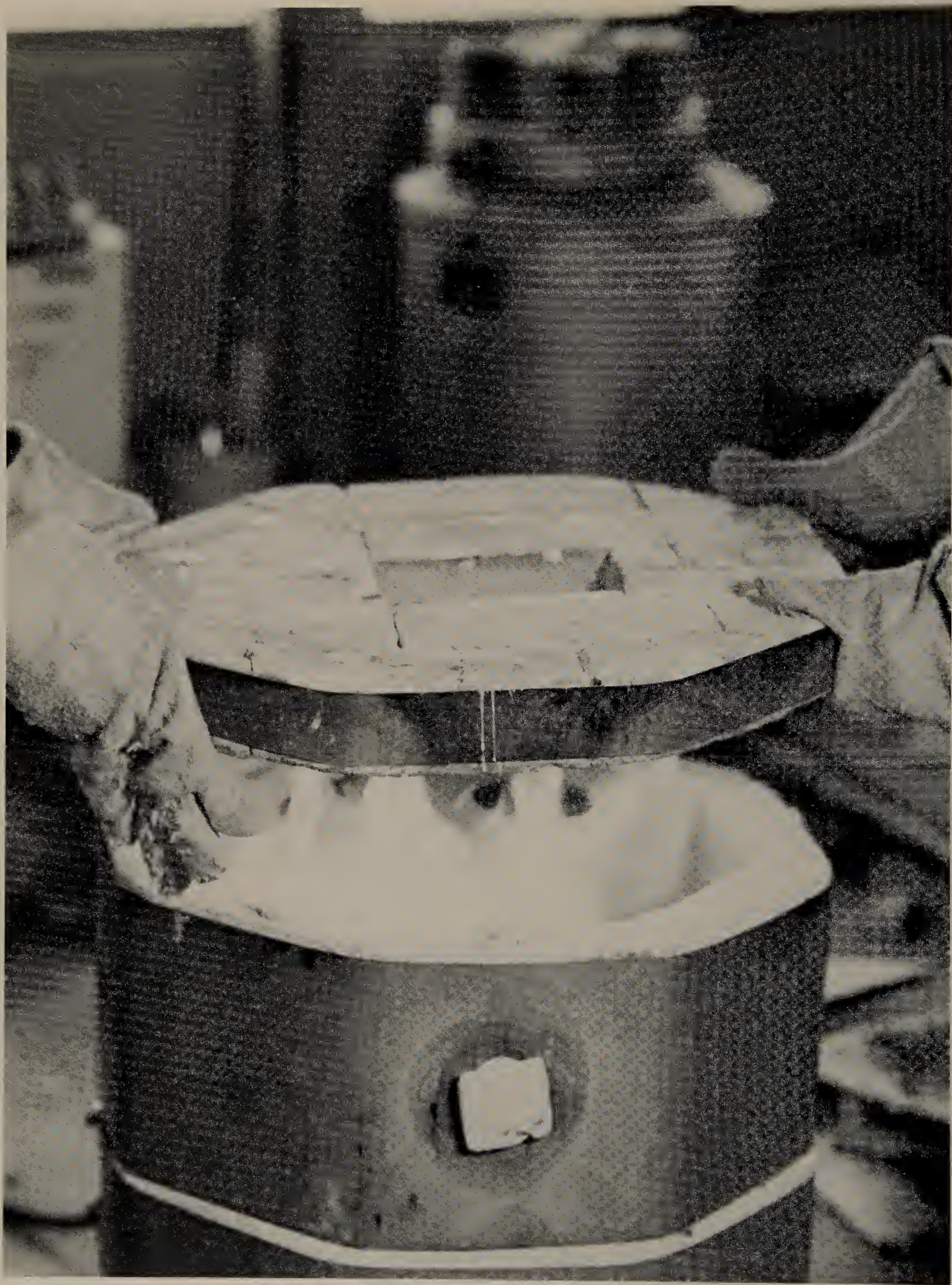
The lid is then replaced and the burners turned higher.
