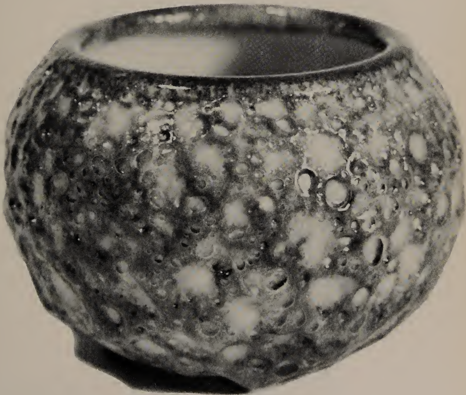
This piece displays an immature copper red glaze. More heat and longer fire would smooth out the surface and produce a mature glaze.
