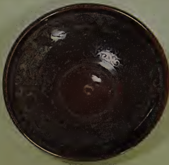
Arabian Luster Glaze T.A.L., colored with pigment 3-3a and fired on schedule T.R. 2, results in an orange-gold luster with iridescence.
