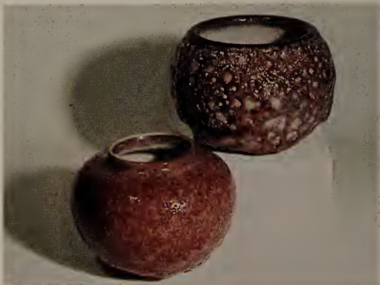
Piece at left displays Copper Reduction Glaze I-12; piece at right, Glaze I-6. Both pieces were fired to cone 9 touching, somewhat below maturing temperature for both glazes.
