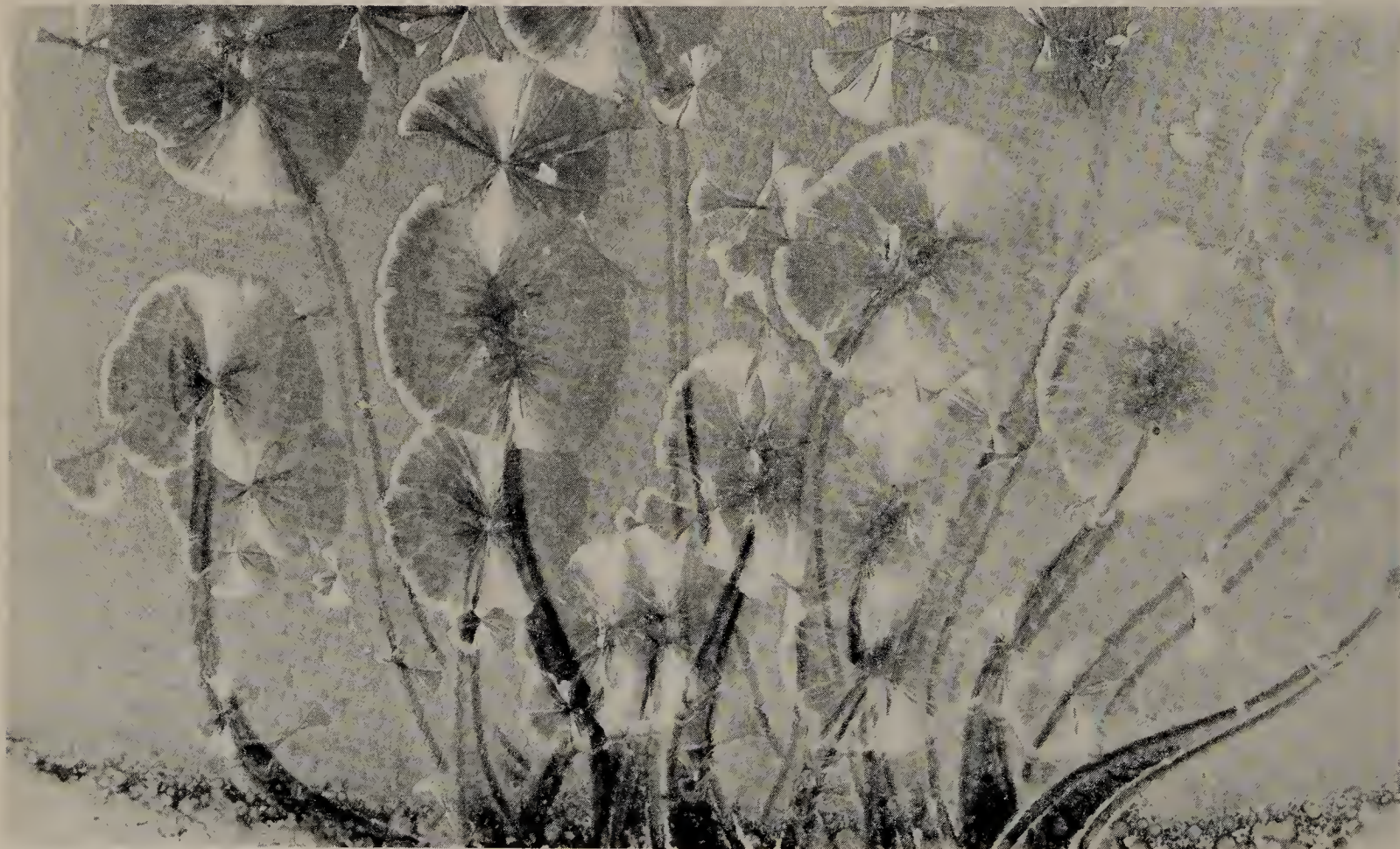
A seeded glaze may produce large crystals in the seeded area, as well as smaller crystals where there has been no seeding. The smaller crystals result from the crystal glaze alone.
