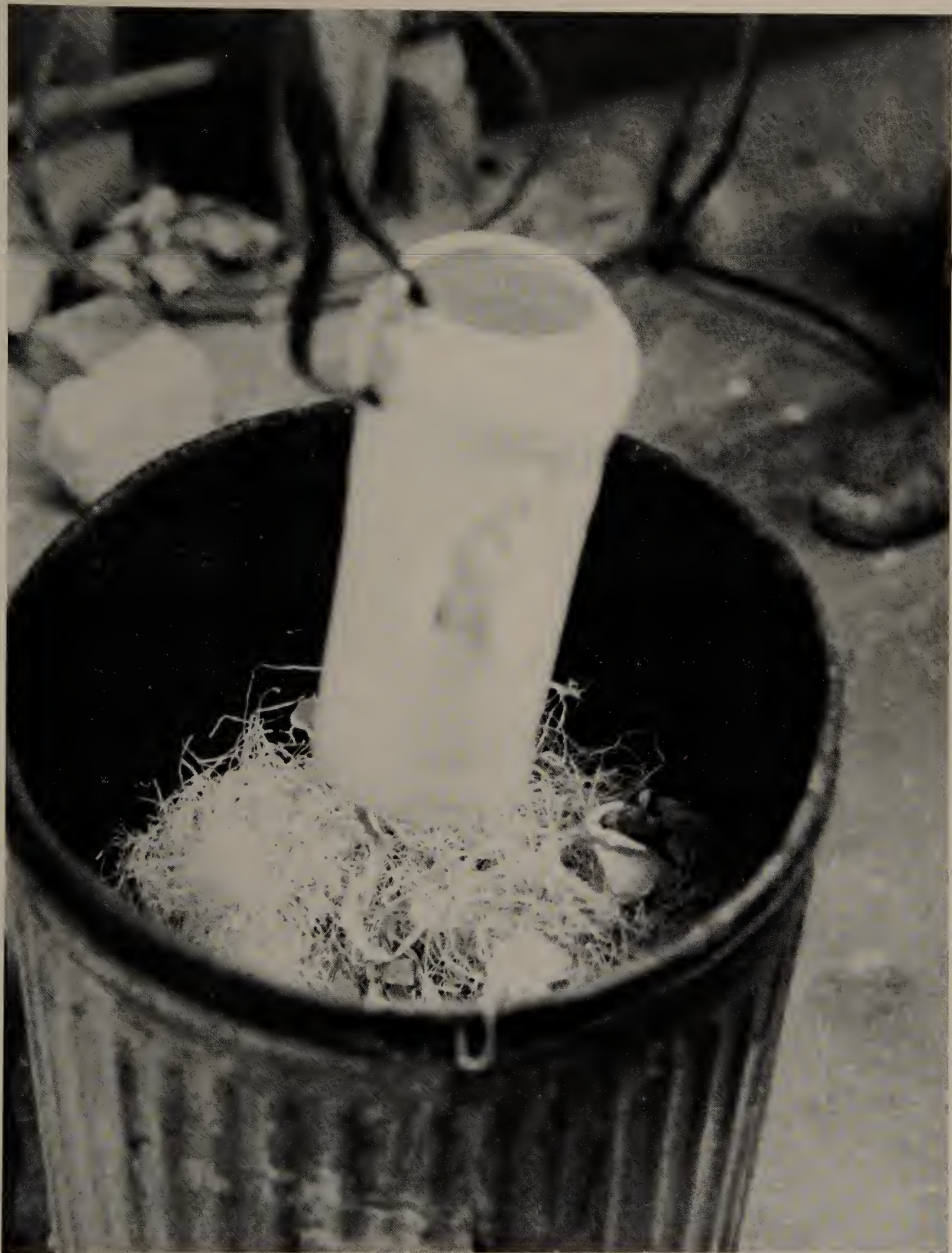
The red-hot ware is removed from the kiln and swung in the air for three or four seconds to set the glaze. As soon as the glaze is set, the pieces are placed in a reduction can partly filled with excelsior and sawdust.
