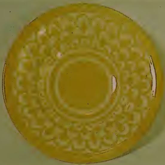
Arabian Luster Glaze T.A.L., colored with pigment 3-3 and fired on schedule T.R. 3, results in a canary yellow luster.
