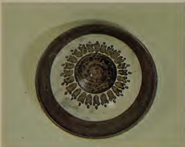
Arabian Luster Glaze R.T.-12, colored with pigment 5 and fired on schedule IV-3, results in a burnt orange and gold luster.
