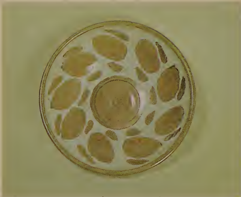
Arabian Luster Glaze R.T.-12, colored with pigment 3 and fired on schedule IV-2, results in a gold luster with abalone-shell iridescence.
