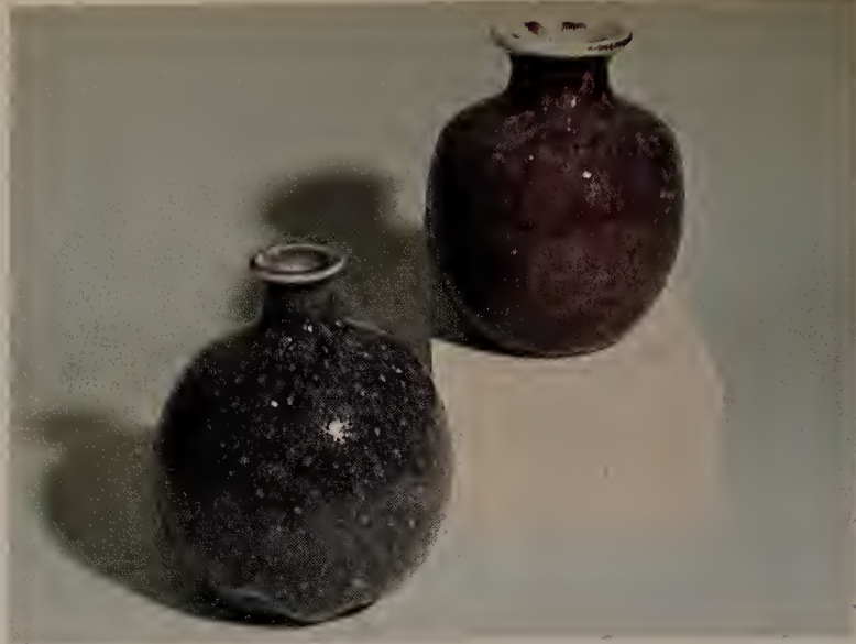
Both pieces were coated with Copper Reduction Glaze IV-14. Piece at left was oxidation fired; piece at right was reduction fired.
