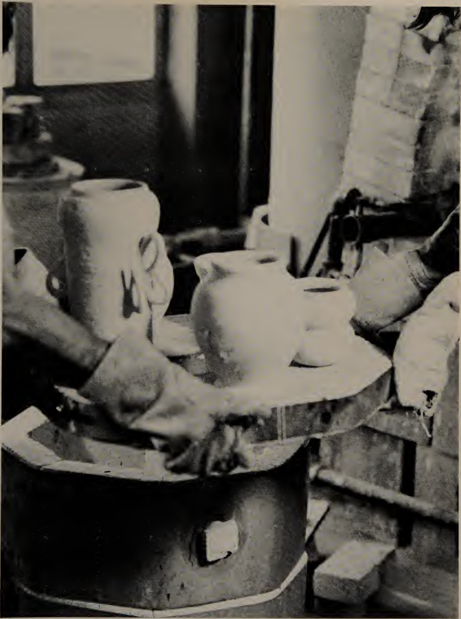
The lid of the kiln is removed, with the pieces in place on top of it.
