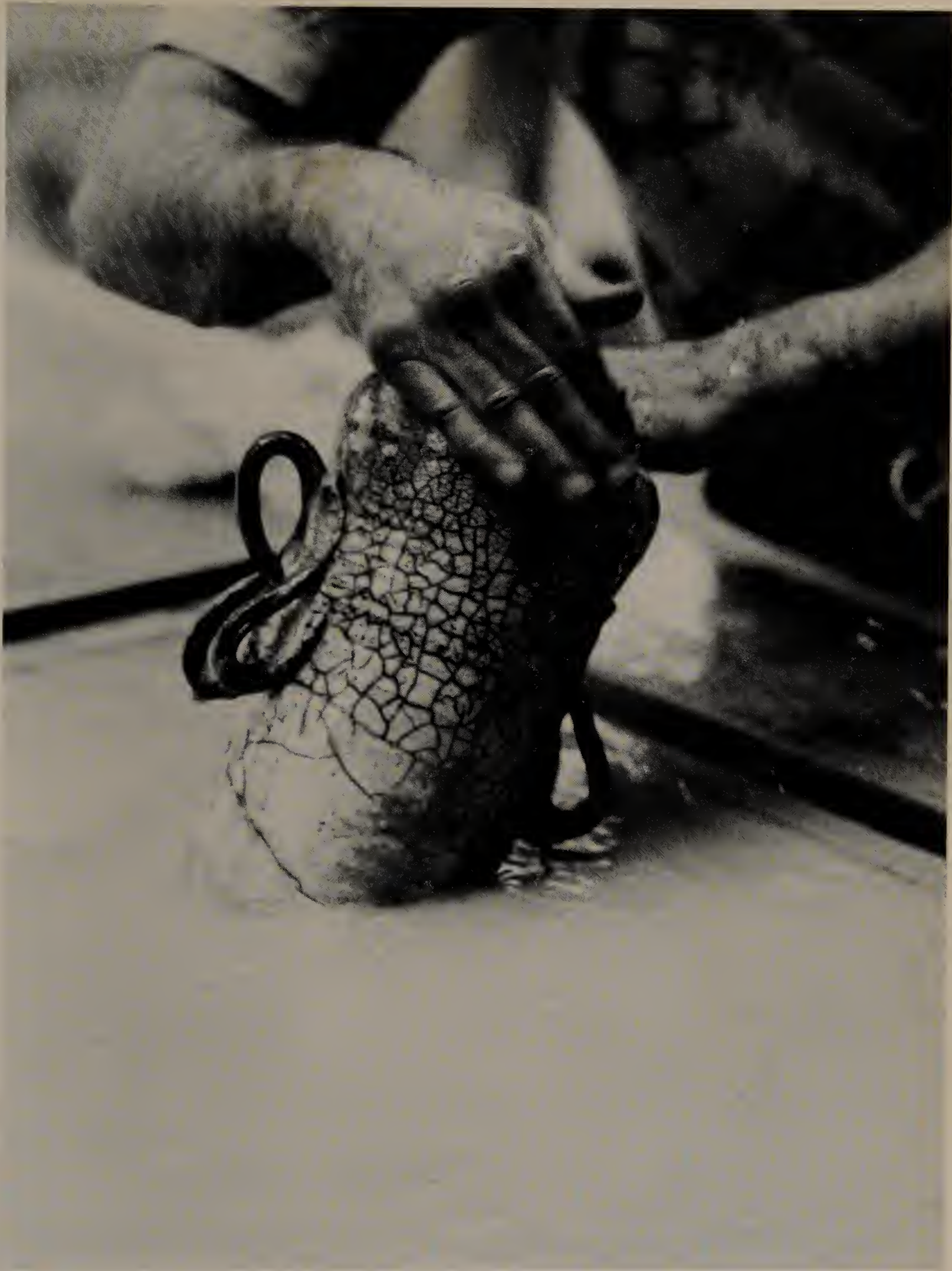
After being removed from the can, the ware is washed to clean the carbon away from the surface.
