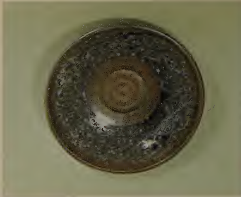
Arabian Luster Glaze R.T.-12, colored with pigment 3-3 and fired on schedule IV-4-a-1, results in a gold luster on mottled gray, with red-violet reflections.
