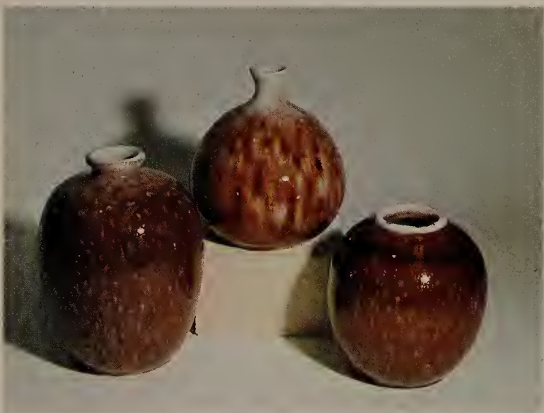
All three pieces were coated with Copper Reduction Glaze IV-2 and oxidation fired; piece in center was fired to cone 11. The other pieces were fired to cone 10 touching.
