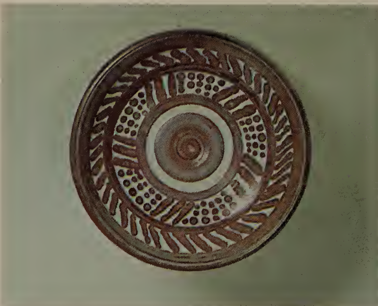
Arabian Luster Glaze R.T.-12, colored with pigment 2-2 and fired on schedules IV-4b and IV-4a-1, results in a red luster with ruby reflections.
