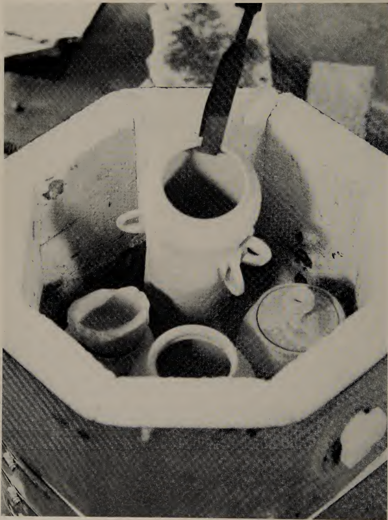
The preheated pieces are then placed in the kiln for firing.
