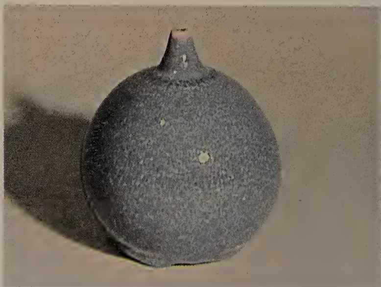
Piece was coated with Copper Reduction Glaze III-8 and oxidation fired.
