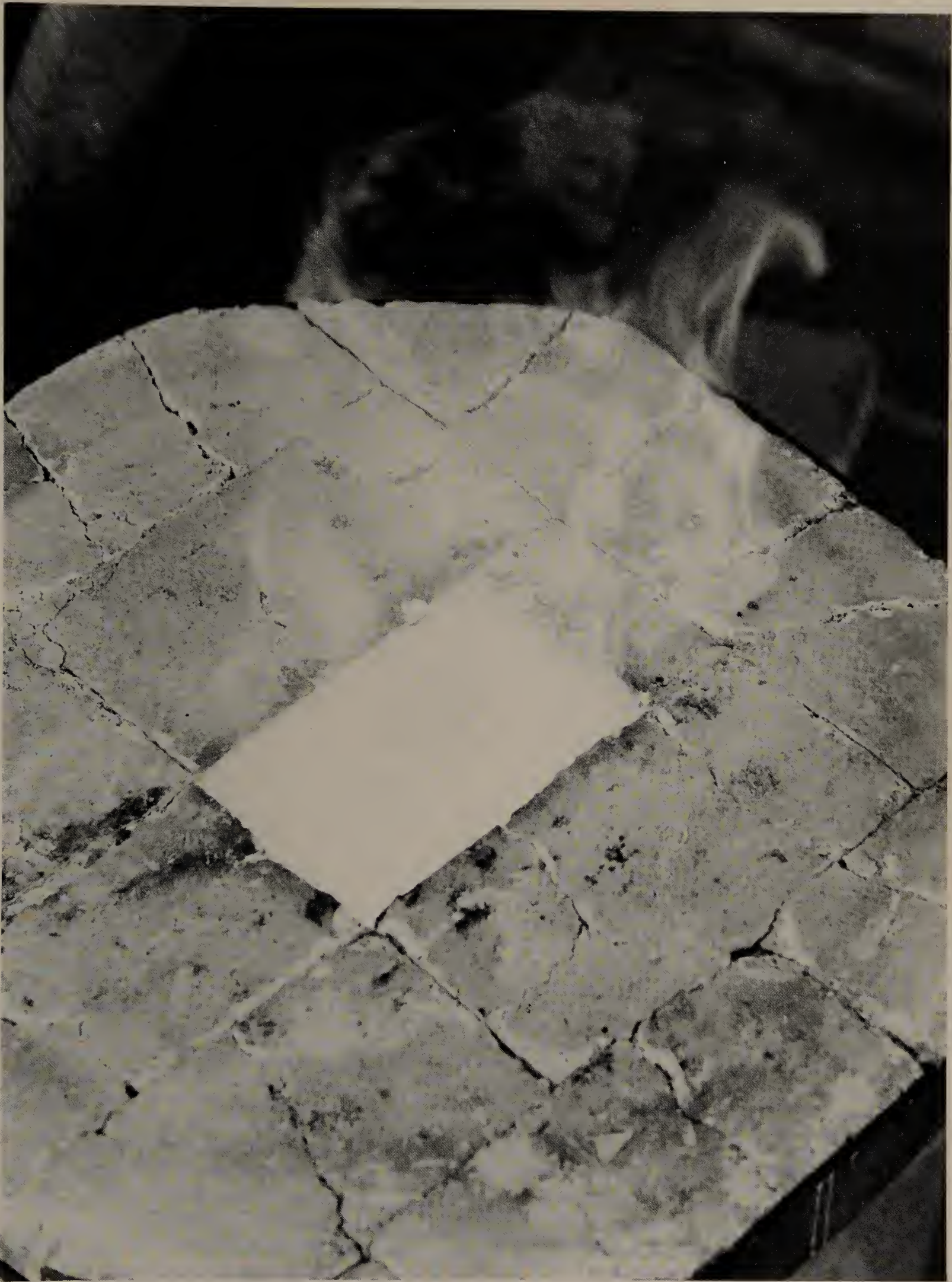
The heat in the raku kiln is gradually increased until the glaze is matured.
