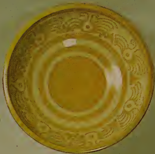
Arabian Luster Glaze T.A.L., painted by Robert Johnson and colored with pigment 3 was fired on schedule T.R. 4, resulting in a canary yellow luster.
