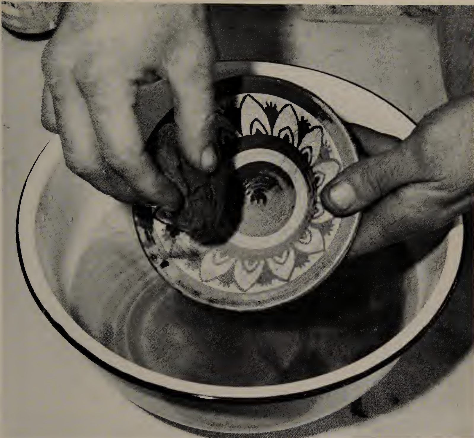
After firing, the pigment is washed off the smoked Arabian luster piece.
