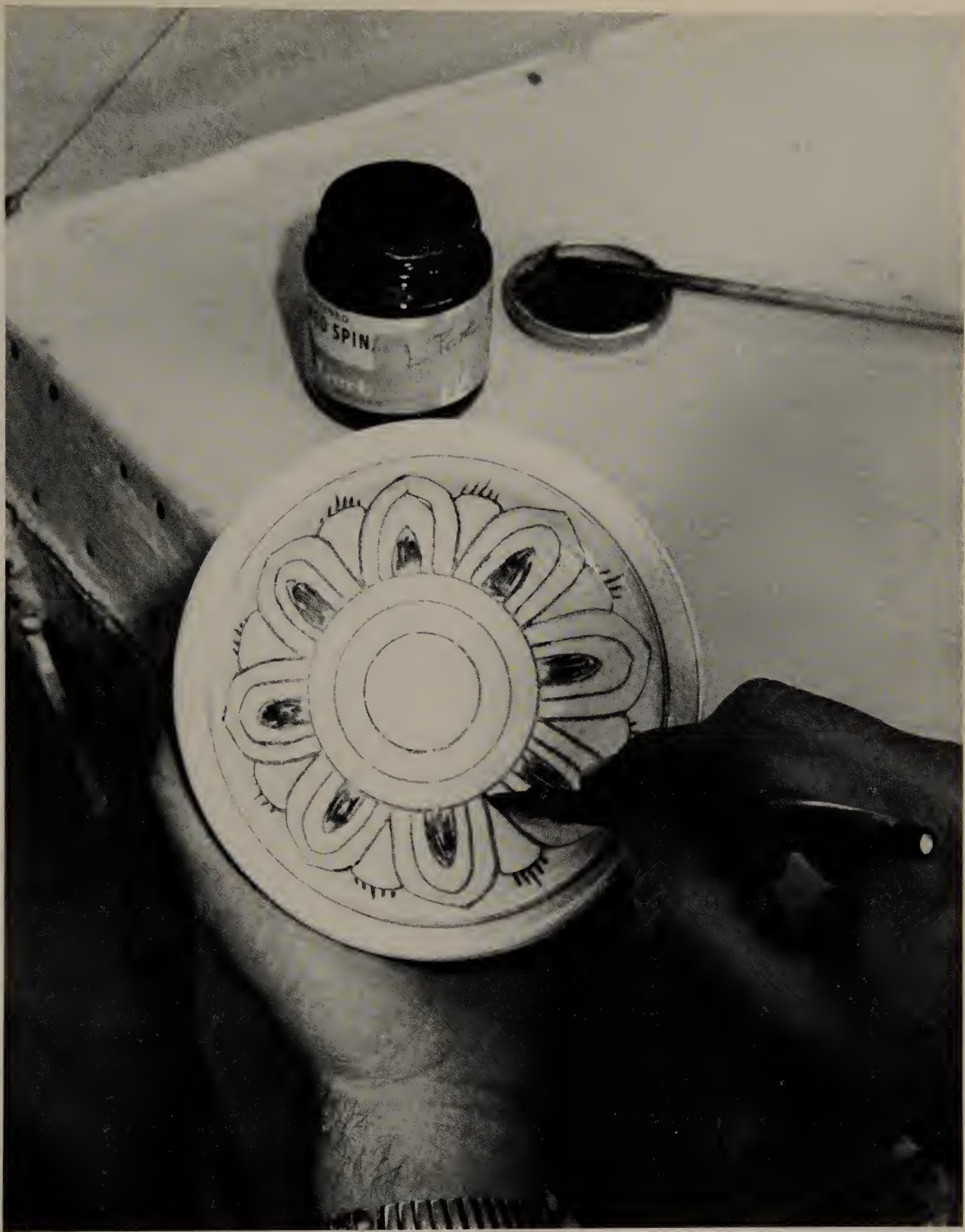
A felt pen should be used for sketching patterns on top of smoked Arabian luster glazes. Demonstration by Robert E. Johnson.
