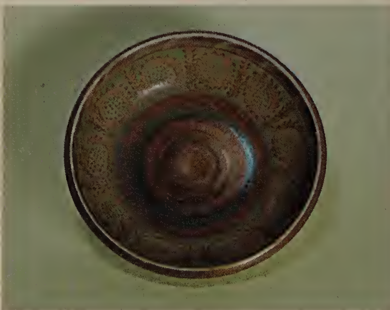
Arabian Luster Glaze R.T.-12, colored with pigment 4 and fired on schedule IV-4a-1, results in an old rose luster with violet reflections.
