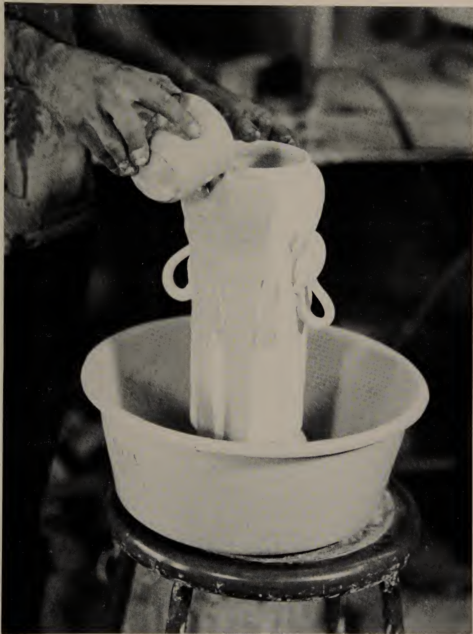
Glaze is poured on the piece in preparation for raku firing.
