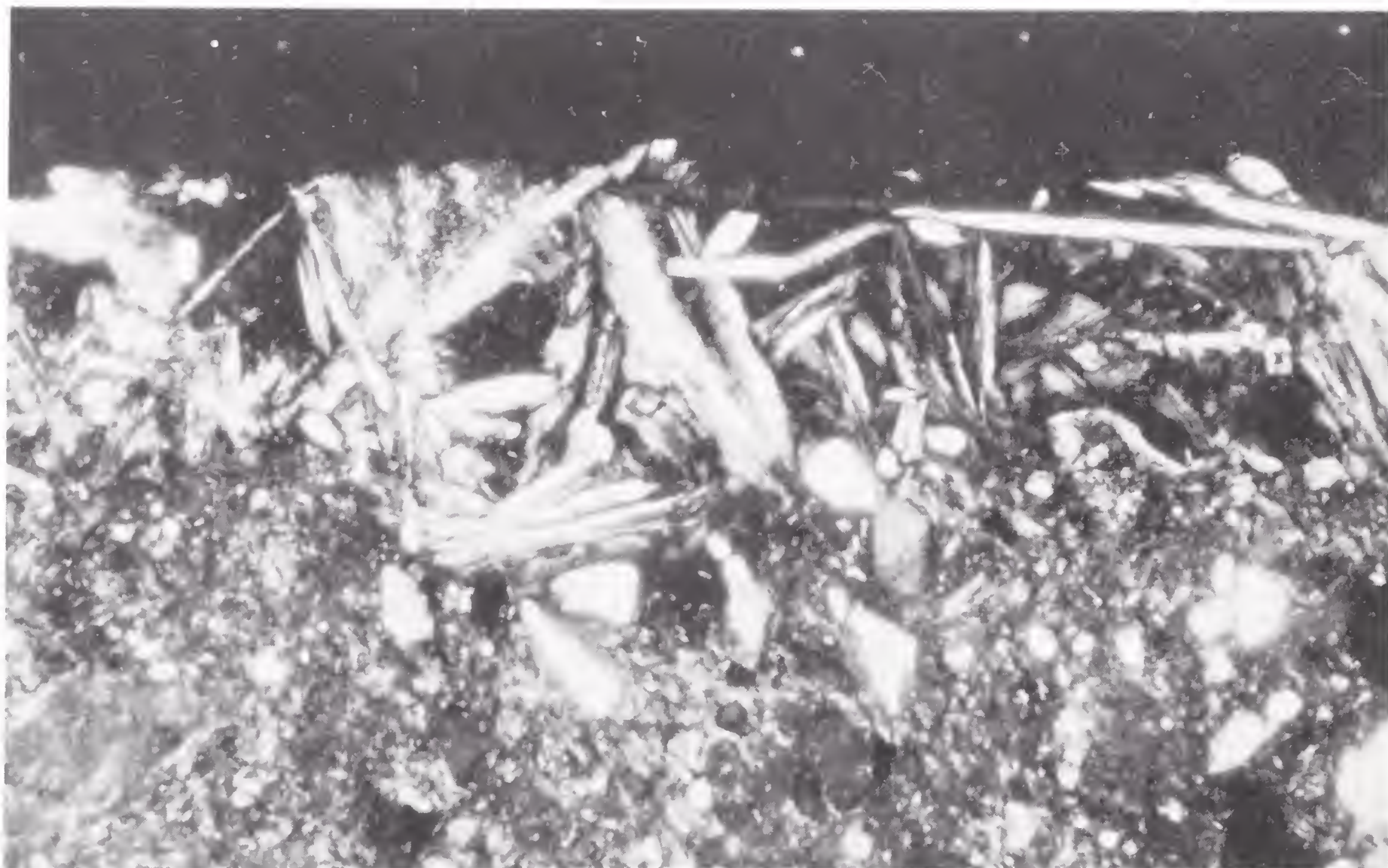
12 Cross section of ash glaze on stoneware. Transmitted light (crossed polars) \times 160 . Notice how integrated the glaze and body have become.
