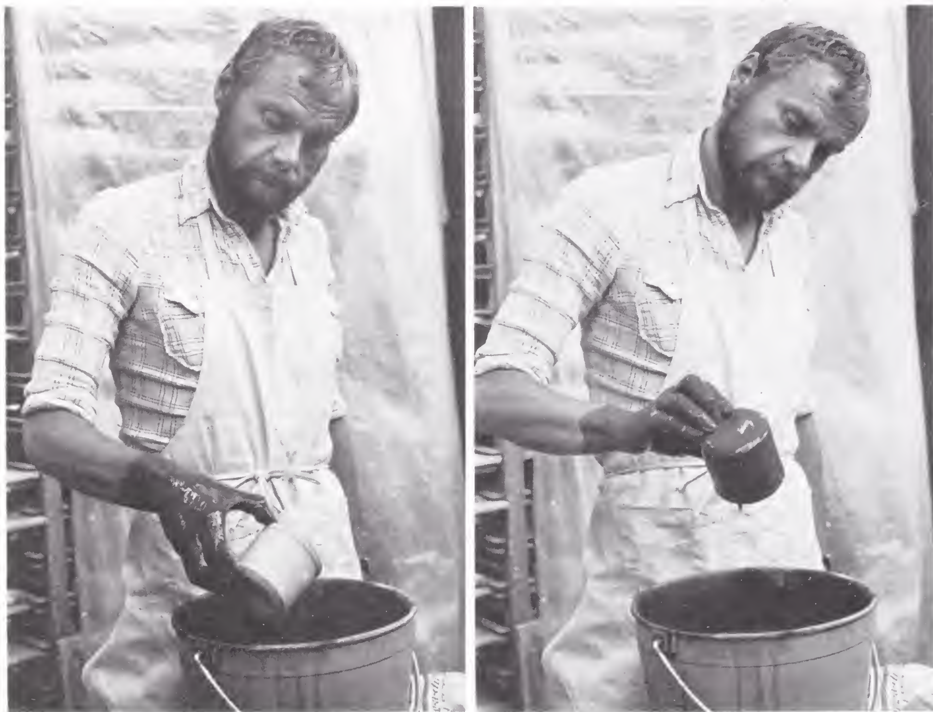
47a & b Dipping the pot inside and outside. a) holding the pot so that no air is trapped inside b) draining the glaze.
