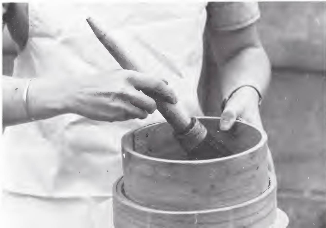
45 Passing glaze through a sieve with a stiff glaze brush. Photograph – Harrison Mayer Ltd.
