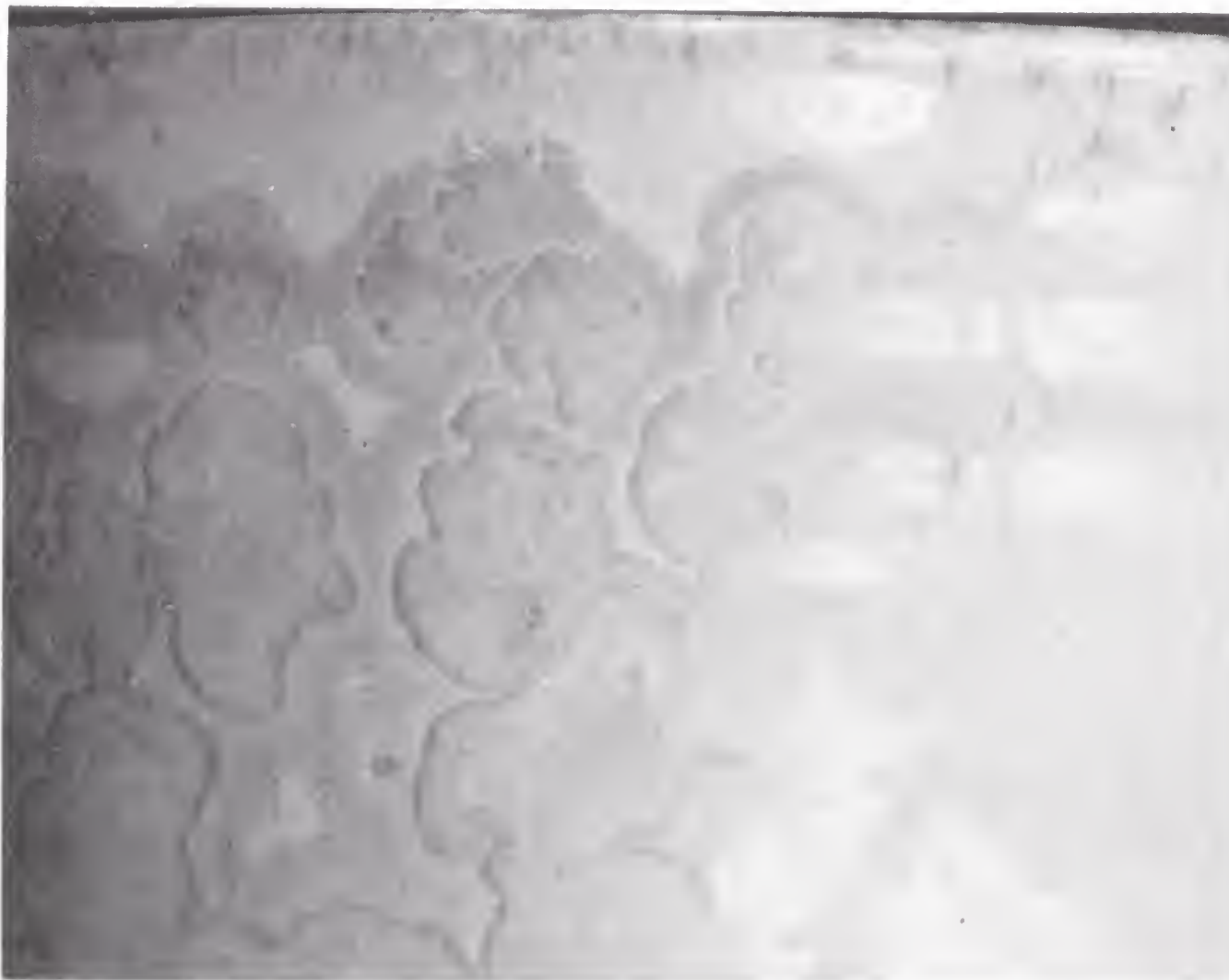
38 Zinc silicate crystalline glaze and porcelain. Creamy white crystals in white background.
