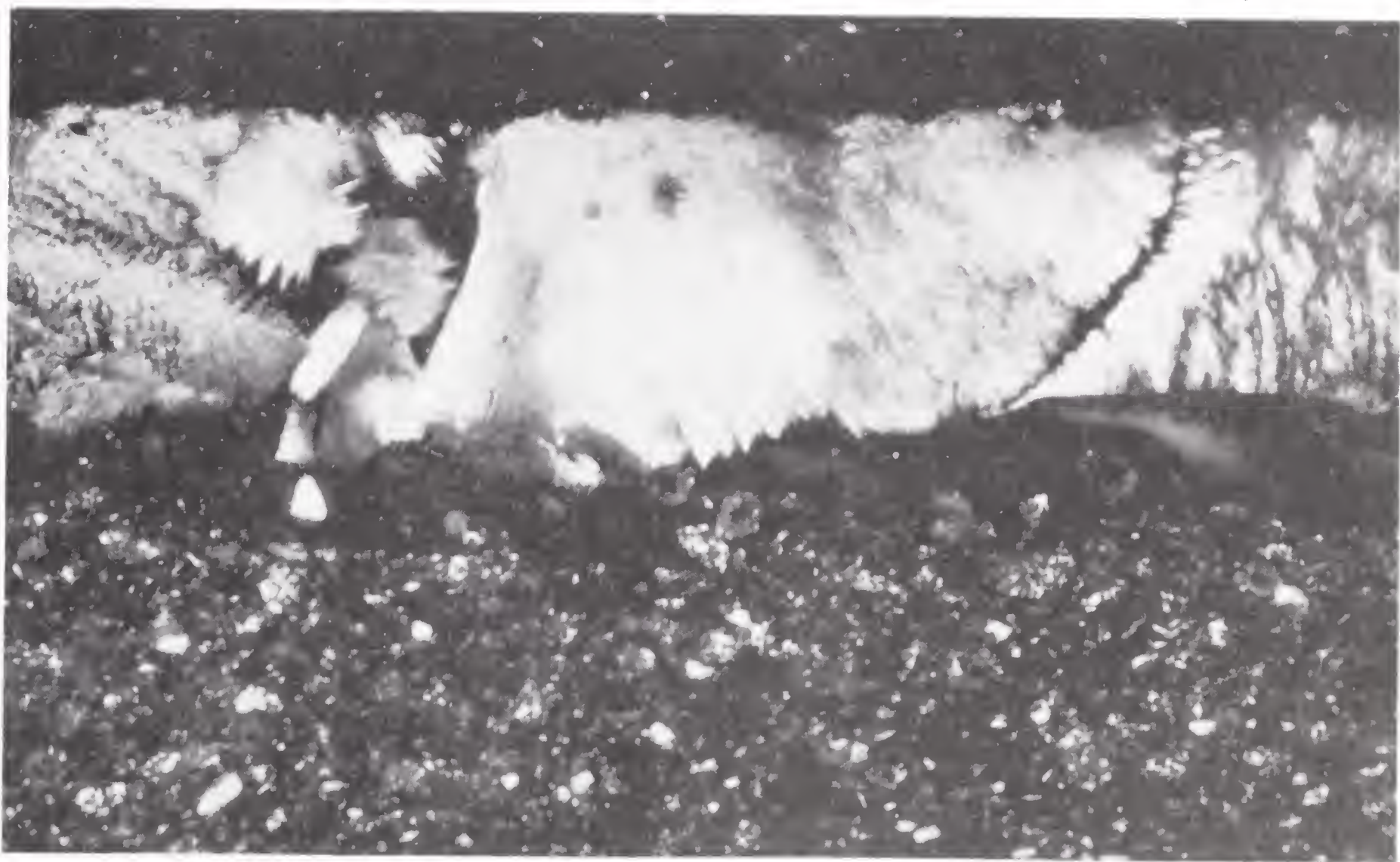
35 Cross section, zinc crystalline glaze (page 163) on porcelain body.
