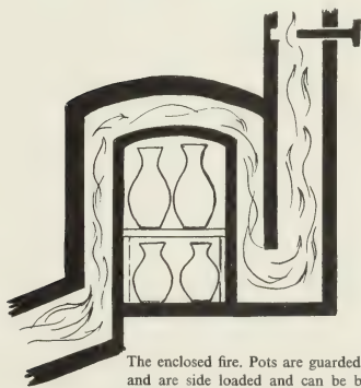
The enclosed fire. Pots are guarded from the flame and can be biscuit-fired or glaze fired in the down-draught. Oxidation and reduction are both possible.
