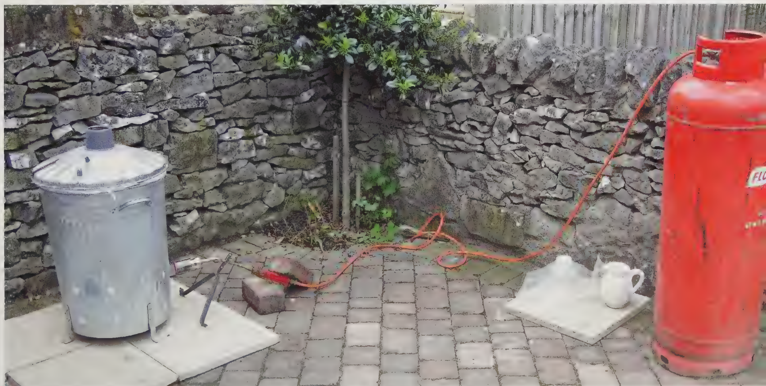
A small raku kiln set up. Photo by the author.
