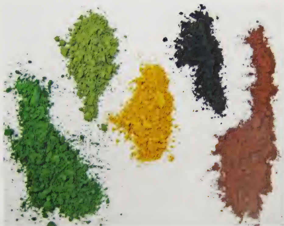
Some naturally occurring colourants: chrome oxide, nickel oxide, yellow ochre, black copper oxide and red iron oxide. Photo by Jennifer A. Siegel.
