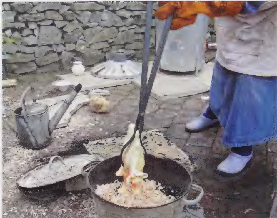
A raku piece is carefully lowered into a metal container containing wood shavings or paper for post-firing reduction. Photo by the author.
