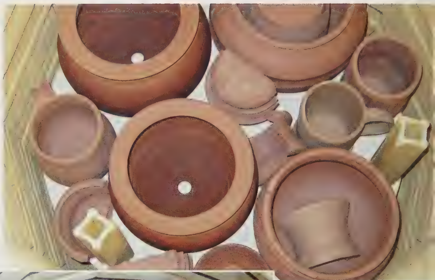
above A loaded electric kiln before a bisque firing, illustrating how pieces can be in contact during this firing. Photo by Jennifer A. Siegel.
