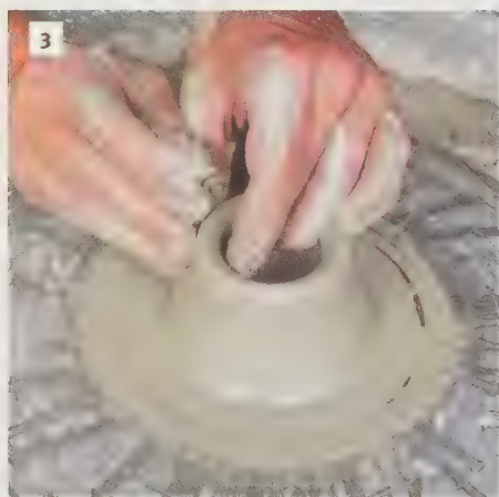
Opening clay to make a spout.
