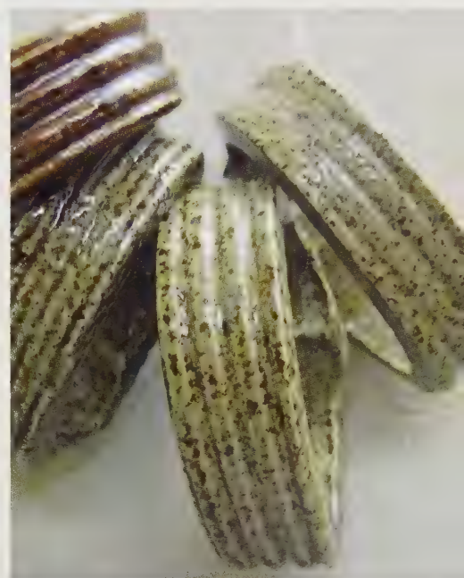
Draw rings removed from a kiln during the firing with an iron rod, used to see how the salt glazing was progressing. Photo by Jennifer A. Siegel
