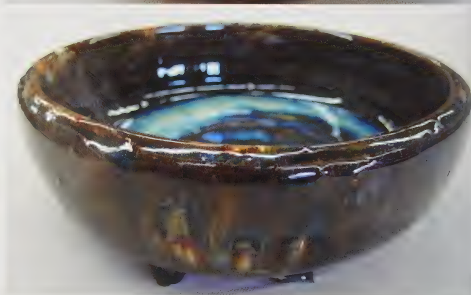
top This pot clearly has some glaze application issues that might best be remedied by washing all the glaze off and starting over. If fired, the fingerprints and cracked glaze will detract from the finish, and the thick glaze will most likely run and stick to the kiln shelf. Photo by Jennifer A. Siegel.
