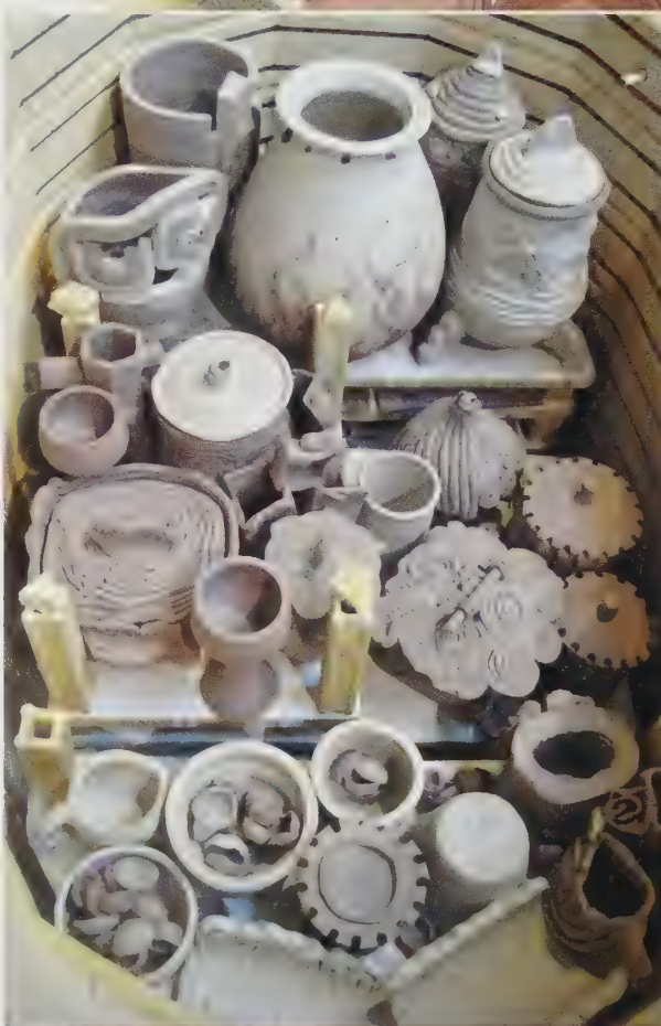
above A loaded electric kiln before a bisque firing, illustrating how pieces can be in contact during this firing. Photo by Jennifer A. Siegel.
