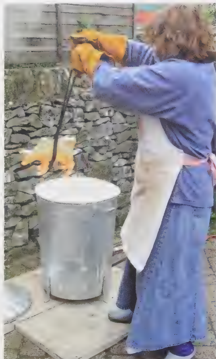
A red-hot piece is removed from the kiln using long tongs. Photo by the author.
