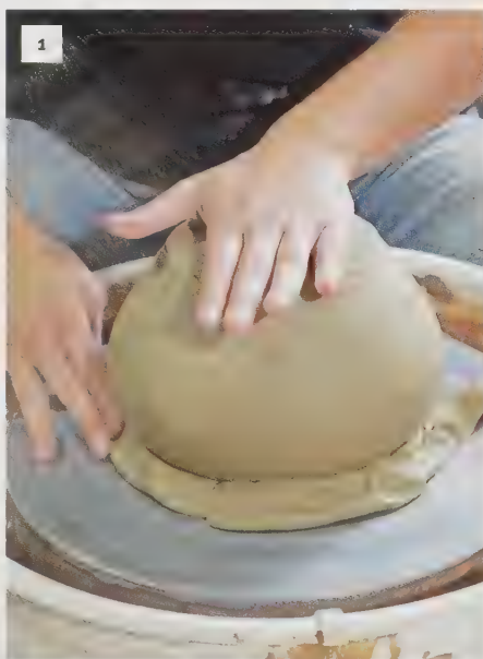
Once centred, pieces must be firmly attached to the wheelhead with soft clay before trimming.
