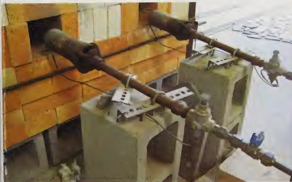
above left An 100 cubic ft (2.8 cubic m) gas-fired salt kiln. Photo by Jennifer A. Siegel
