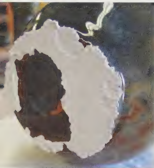
above This glaze has been applied too thickly, and has also not been wiped off the bottom prior to firing. During the firing, the glaze has melted and stuck to the shelf. Photo by Jennifer A. Siegel
