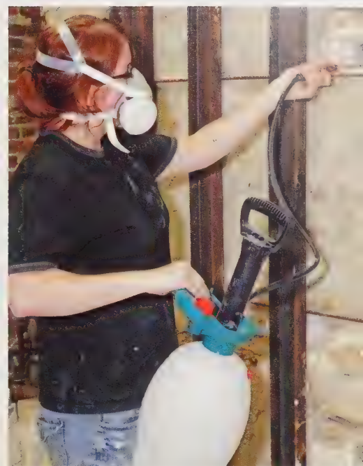
An aqueous solution of salt and soda being sprayed into a gas kiln.
