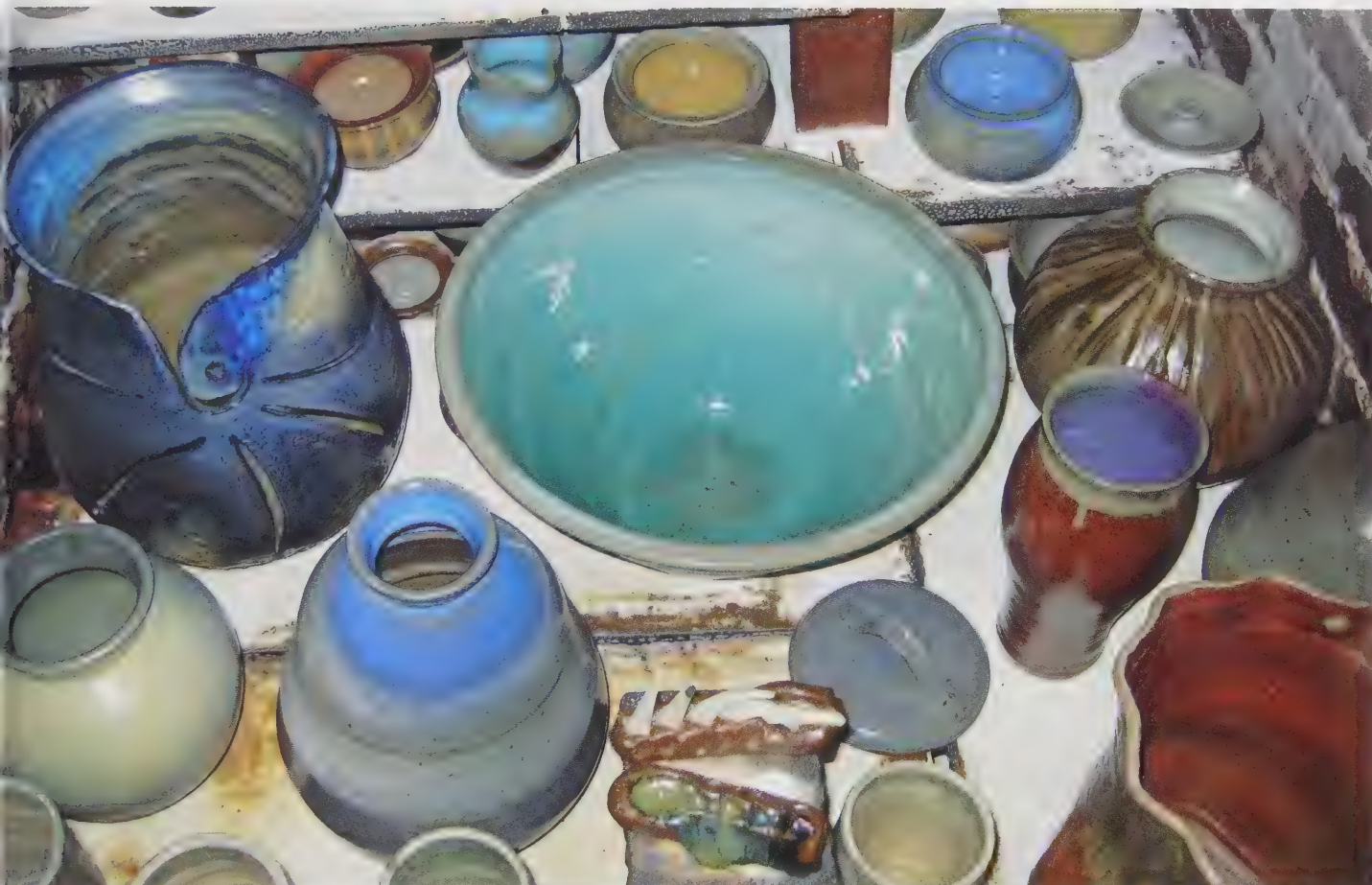
The cone packs in this kiln after firing can be seen in the bottom middle of the image. In the cone pack nearest the bottom of the image, the cones have completely melted and turned to glass. Photo by Jennifer A. Siegel.
