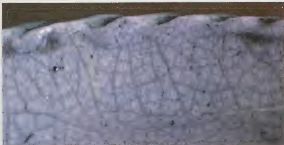
above left Detail of a crawling glaze. Crawling glazes can add an interesting surface, especially to sculptural work. This effect is usually created by applying a thick layer of glaze with an over-abundance of fine particled clay (ball clay or bentonite) in it. This clay layer usually cracks during drying, which then results in crawling during the firing. Photo by Jennifer A. Siegel top, right Crazing can pick up the carbon during the raku process. Photo by the author bottom, right Crazing in a glaze shows up as little cracks in the surface.
