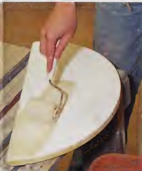
Kiln wash or bat wash being applied to a kiln shelf. This can be purchased already mixed or you can make your own.
