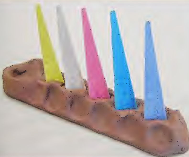
A cone pack before firing. Photo by Jennifer A. Siegel.
