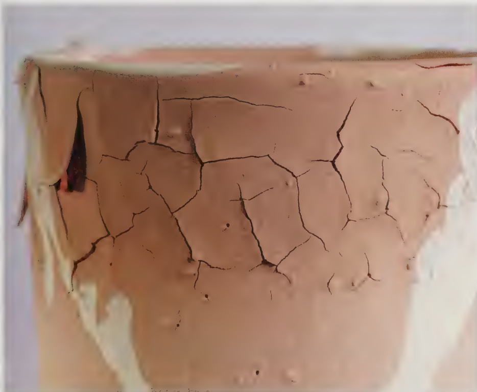
Glaze applied too thick will sometimes crack. This glaze will need to be washed off and reapplied.
