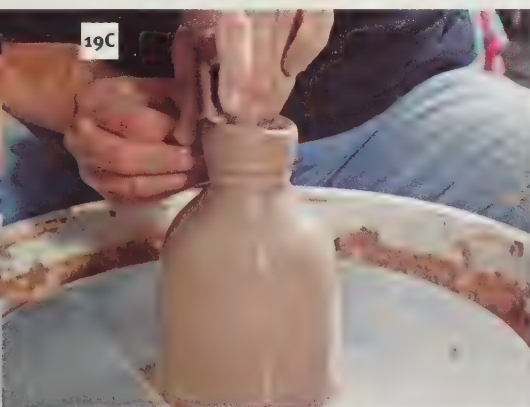
Smoothing out the top rim having collared in the neck.
