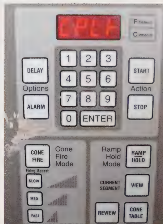
Keypad for electric kiln digital controller. The controller allows the user to use pre-set schedules or to develop and save their own.
