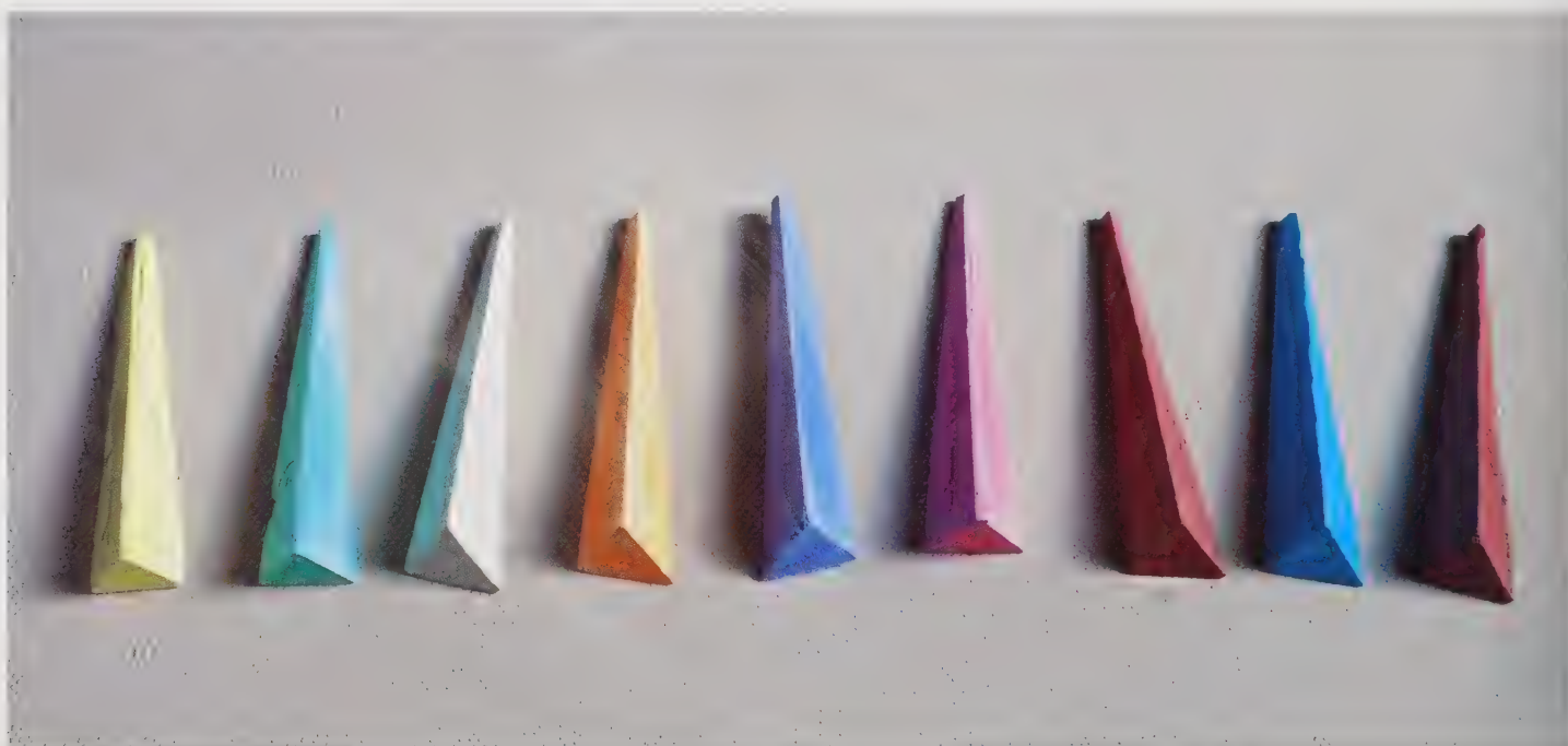
Pyrometric cones are colour-coded to help distinguish between them during handling.
