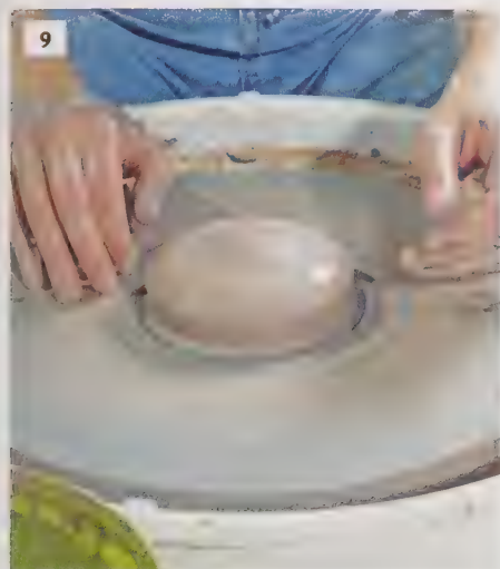
An example of well-centred clay ready to open up.
