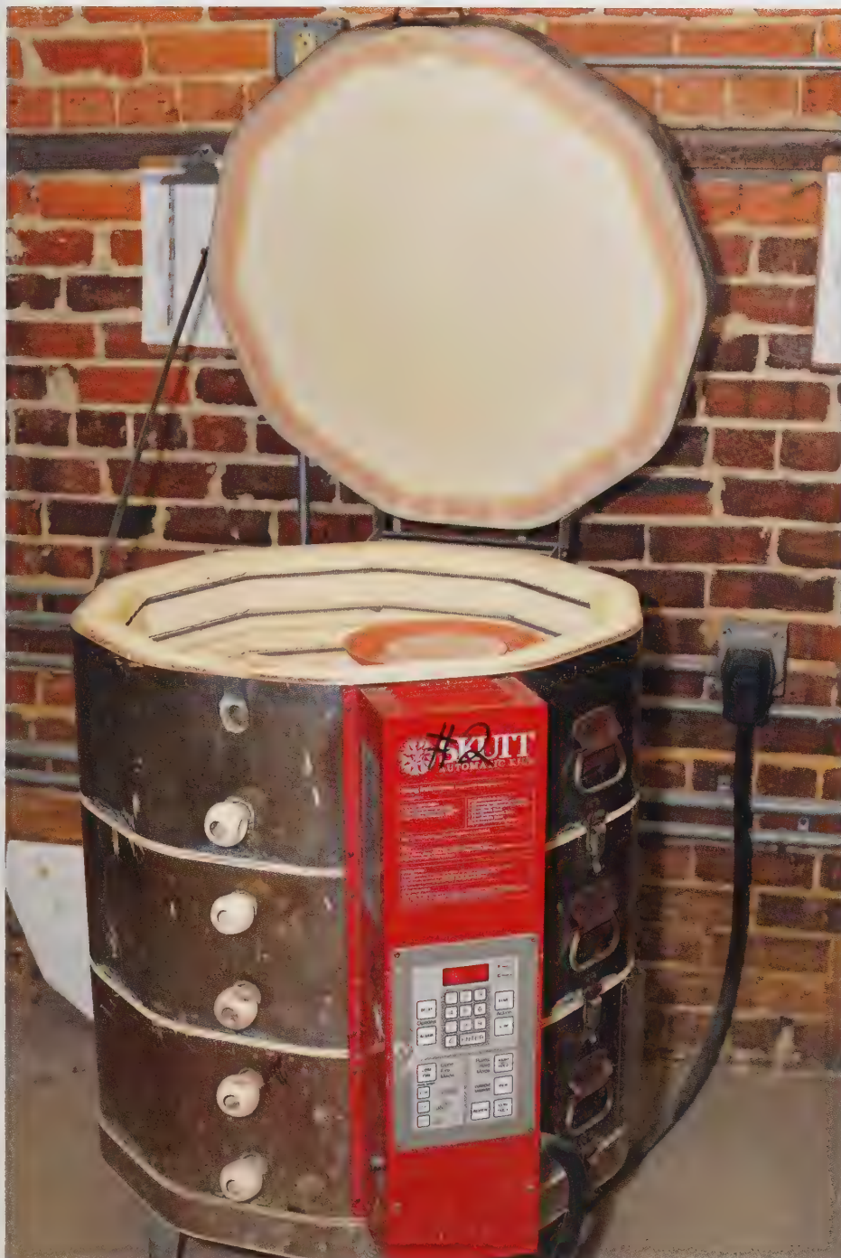
A top-loading electric kiln with programmable digital controller.
