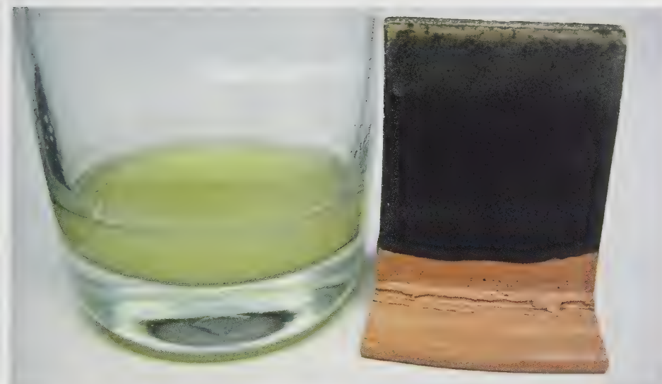
Unstable glazes will leach colourants into food. This image shows a tile that has leached colourant after contact with lemon juice. Photo by Jennifer A. Siegel.
