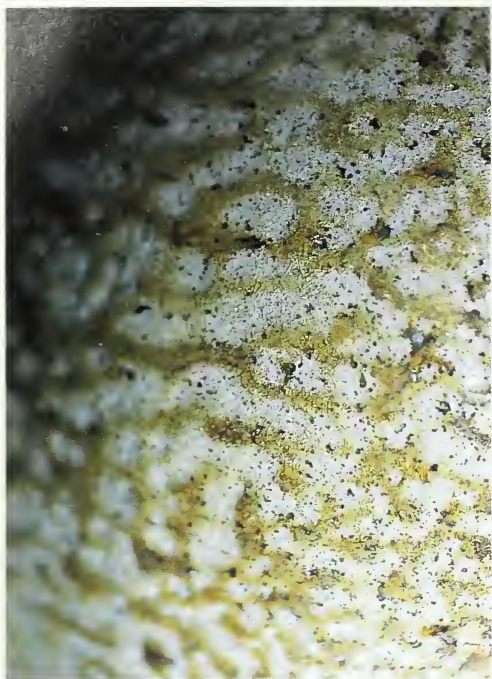
Heavy soda on high iron body.
