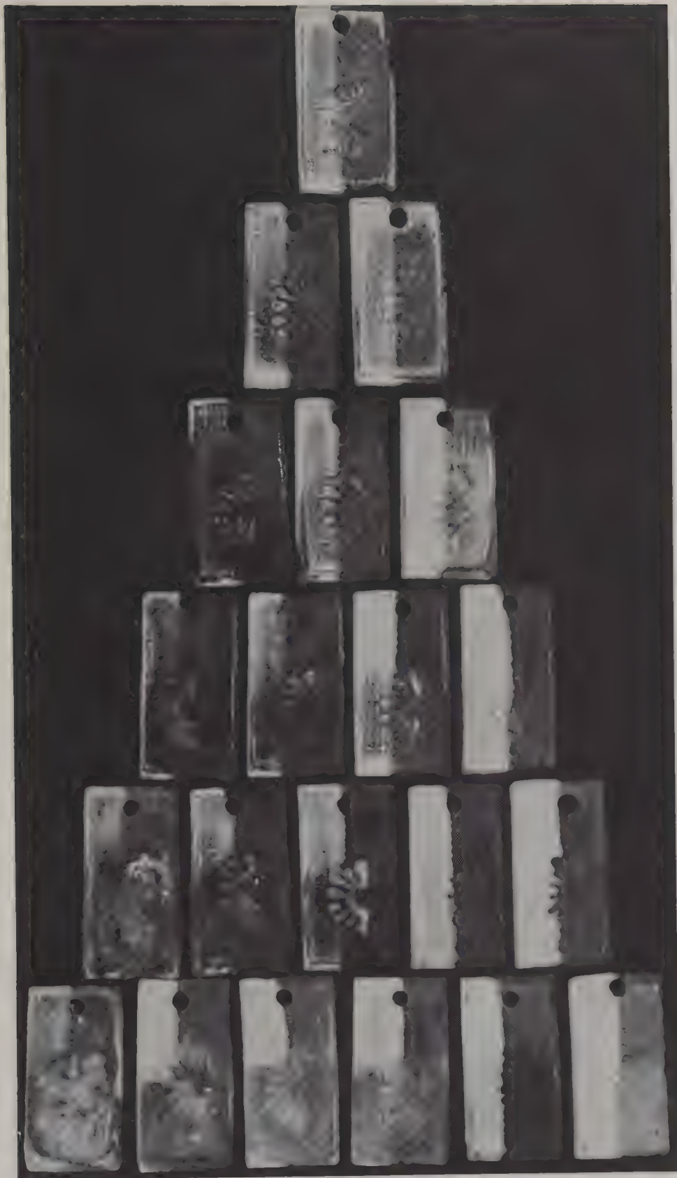
8-2. 21-point triaxial blend test.
