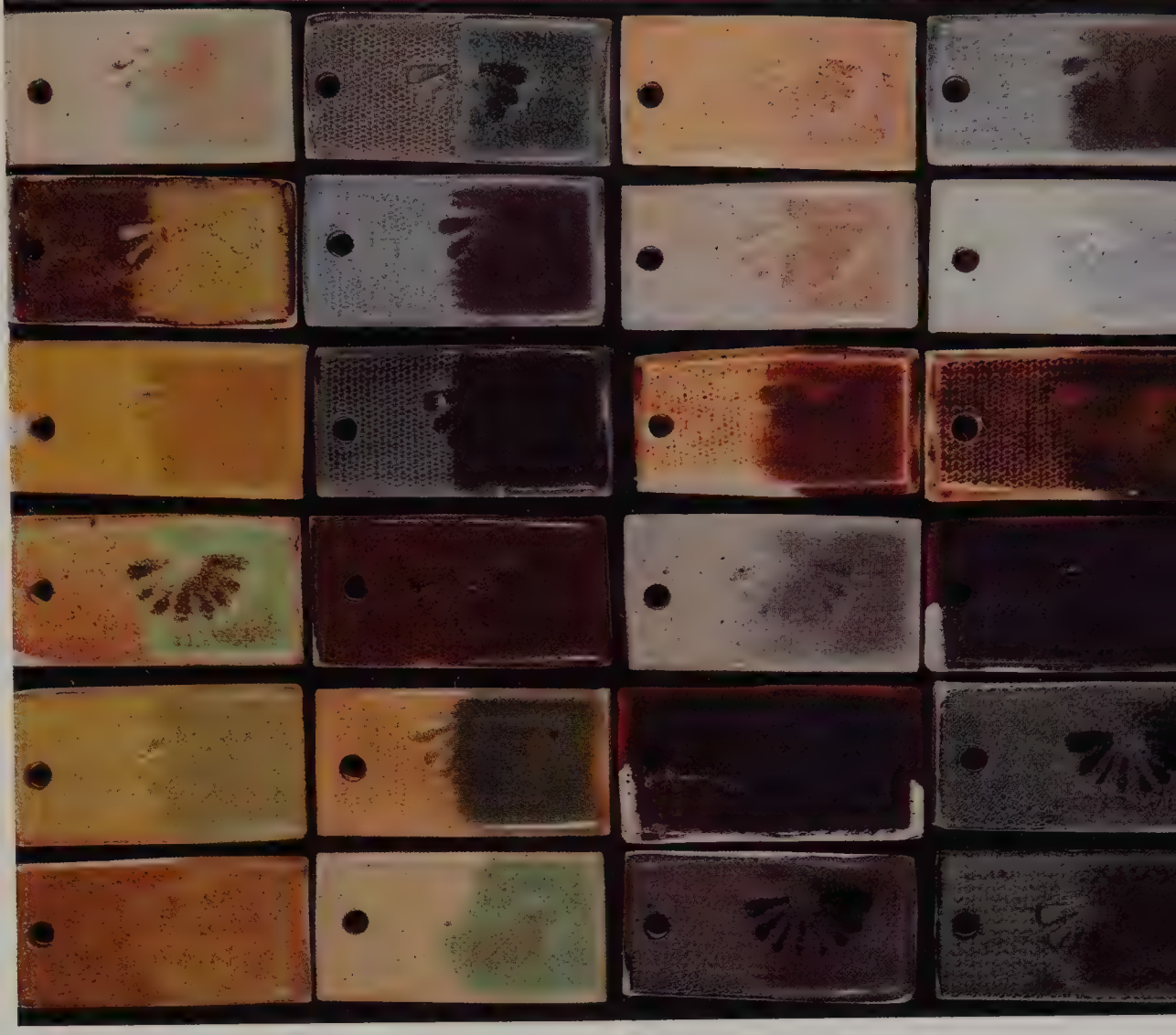
Glaze test 10: Color variations from cross-blends of nickel, manganese and cobalt in various glaze bases.
