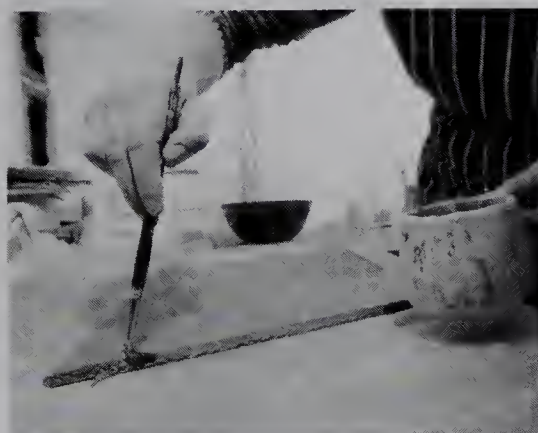
9. Liquid slip is brushed onto the scored surfaces to be joined together, to assist adhesion.
