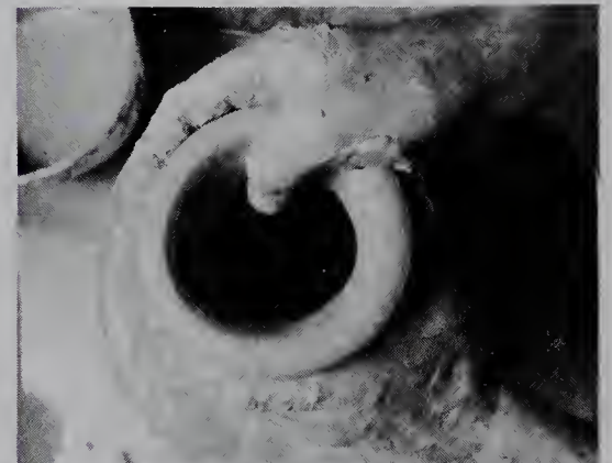
2. The neck of the pot is collared by the left and right hand while the crook of the right thumb applies downward pressure to keep the top level.
