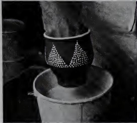
Dipping glaze 1. A large container is filled with glaze. The pot can be held steady with glazing tongs or by bracing the fingers inside the neck of the pot to hold it firm.
