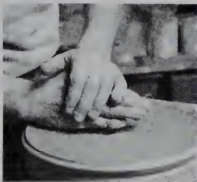
4. The inside dimension of the plate is flattened with the edge of the hand and a steadying grip from the right hand.
