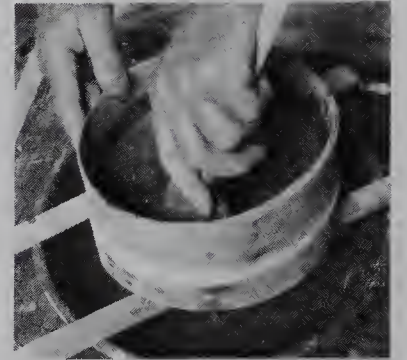
6. The slip is sieved through a 100-mesh sieve (as shown) using a rubber kidney to push the slip through and clean as much as possible from the sides.
