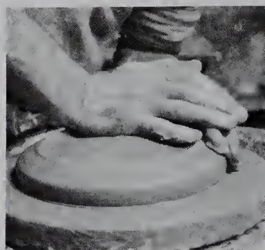
2. Pressure is applied to the clay with the palm of the hand in order to spread the clay out as the wheel revolves.
