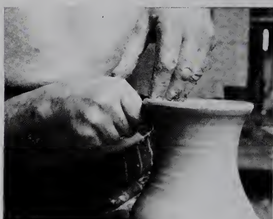
11. The outward flare at the top of the vase is shaped with the inside flat of the finger tips. Gentle thinning, as well as shaping, can continue up to this point.
