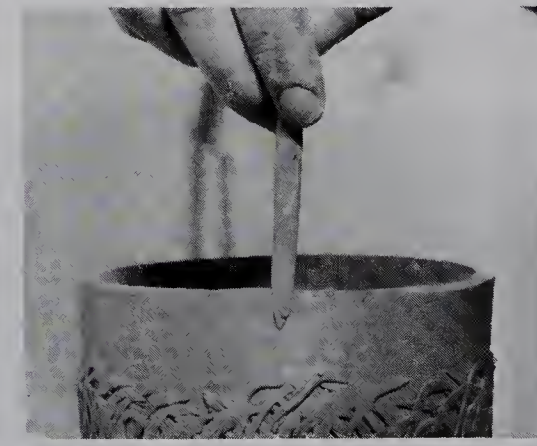
14. A boxwood modelling spatula is used to smooth and compress the join. The pot should be allowed to dry slowly to prevent cracking or springing of the join during firing.
