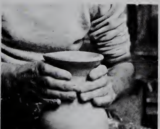
12. The top of the vase is collared to increase the narrowness of the neck before further shaping with the fingertips.
