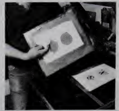
3. A paper stencil is fixed to the back of the screen for printing the covercoat over the transfer. The paper is held to the mesh of the screen by the tacky covercoat.
