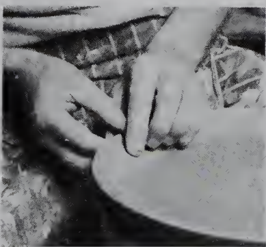
6. The rim is thrown and shaped from the surplus clay around the edge of the plate.
