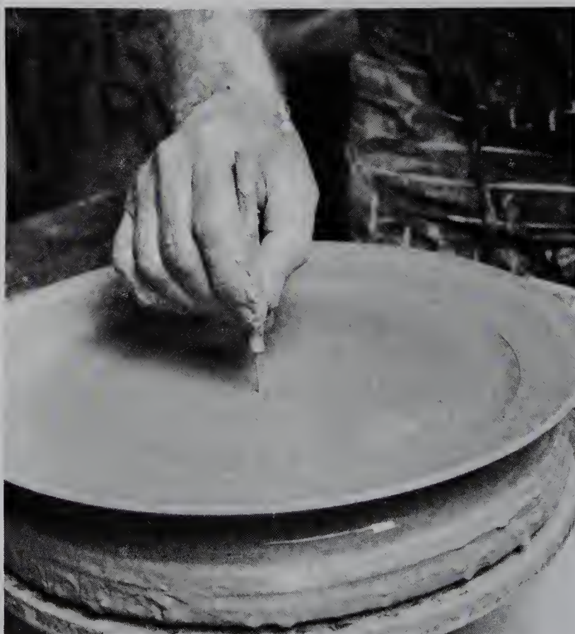
8. After gauging the plate's thickness with a needle, lever the bat from the wheelhead with a metal tool or the end of a mild steel turning too. The plate
