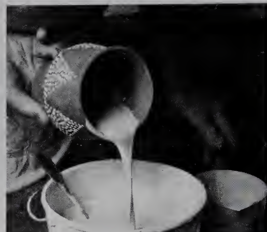
To glaze the inside of a pot, some glaze is poured in, swilled around and any excess poured away. A pot to be dipped in glaze should be glazed on the inside first.
