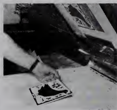
8. Lift the screen and remove the tile.
