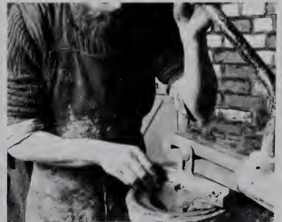
3. Jollying in progress. Keep the template dampened during use.
