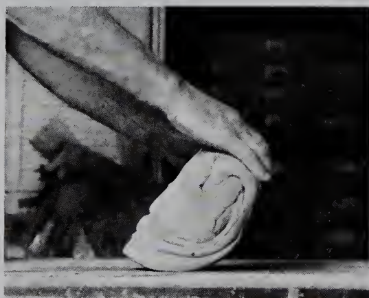
3. The lump of clay is lifted from the back and pulled forward to a vertical position.
