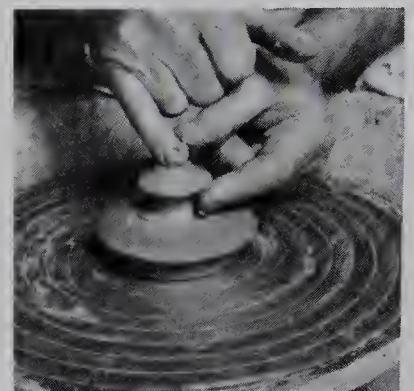
4. The final shaping of the knob is done with the little finger, while the fingers of the other hand support it as it revolves on the wheel.
