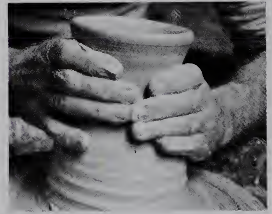
5. The pot is collared using the thumb and palms of both hands for complete control.
