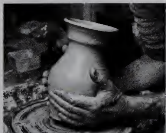
17. The pot is lifted from the wheel with dry hands before placing it on a board or bat to dry.
