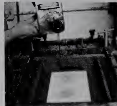
4. Covercoat is poured onto the screen before printing. Keep the can be closed when not in use and only use a little at a time, as it dries very speedily.
