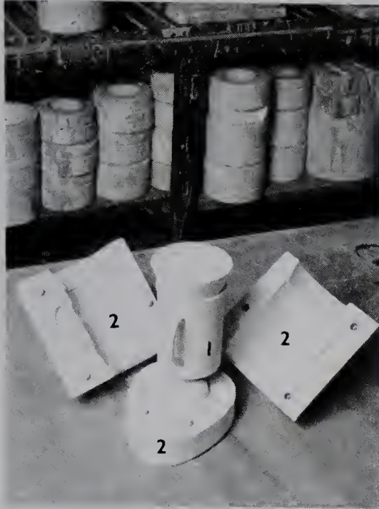
A solid plaster model (1) and its three-section block mold (2), consisting of a base and a two-section body mold. This block mold can become a working mold for further reproductions, the model being redundant.
