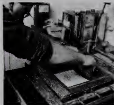
5. The covercoat is printed through the paper silhouette.
