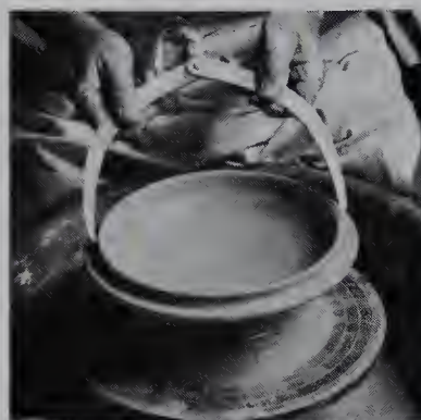
Using calipers 1. A pair of calipers is used to check outside diameter of the rim to ensure that the lid snugly fits the aperture of the pot.
