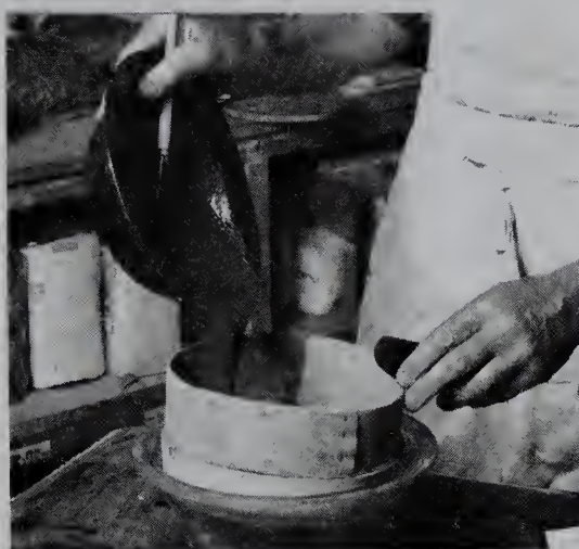
3. The mixture is sieved through a 100-mesh sieve.
