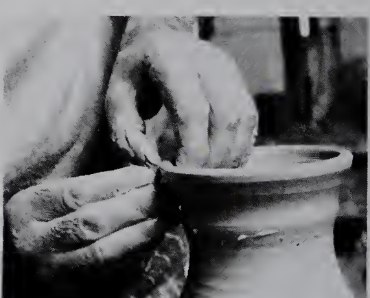
14. As the wheel revolves slowly, the final shaping and thinning of the top of the vase is done, using the tips of the fingers.
