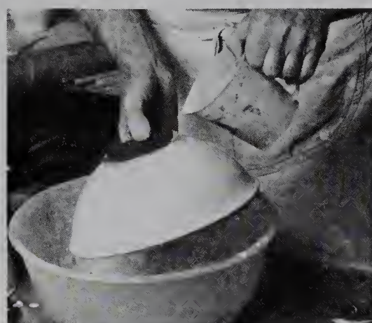
2. The glaze is poured over the pot until the surface is completely covered. Any finger marks can be touched up later.
