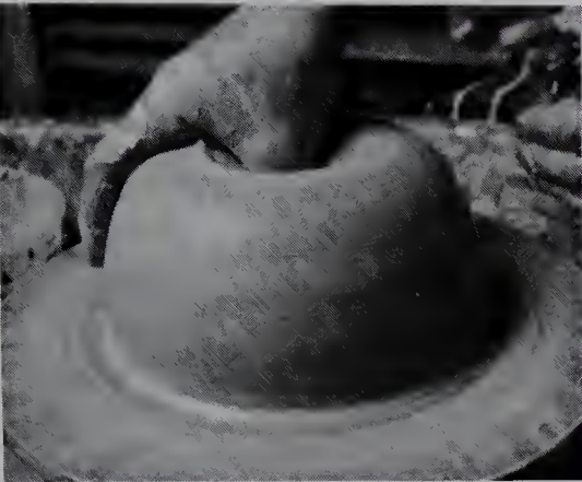
9. The pot is further opened by inserting a thumb.
