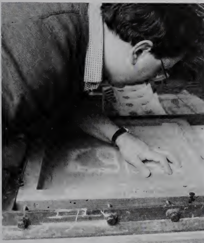
2. Lower the screen and check the registration. This is vitally important if you are going to print more than one color. You can make registration marks on a
