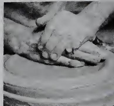
3. The clay is flattened with pressure from both hands.
