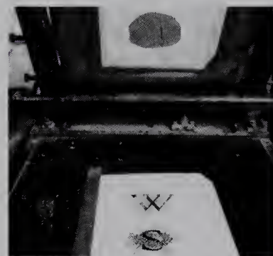
6. After printing, the coverage and section of the stencil on the screen is clearly seen.
