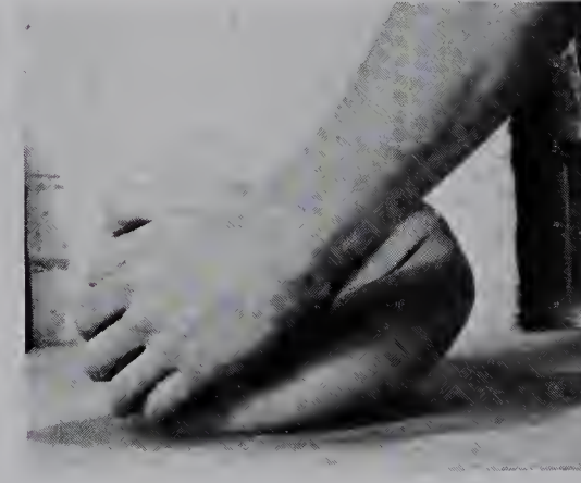
2. After completing the first stage of spiral wedging, lift the clay and repeat the process on the other side.
