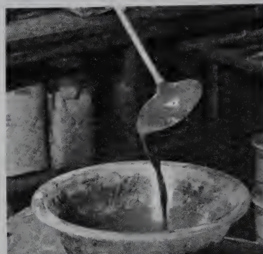
5. The final consistency of the glaze should be that of thick or thin cream, according to the thickness of glaze required and the method of applying it to the ware.
