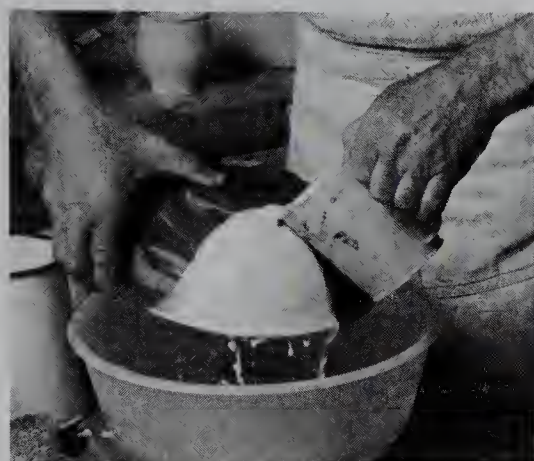
Pouring 1. A small jug is used for pouring the glaze and a larger vessel for catching the drips. Pour into the inside first, holding the article at an angle, so the glaze does not fill the footring.
