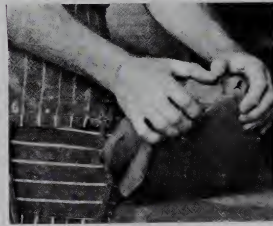
4. The clay is lifted from the right and twisted through 90°. It is then rested on the edge of the bench, cut again and the sequence repeated until the clay is thoroughly mixed and homogeneous.
