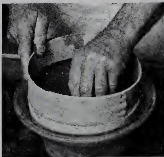
4. You will have to help the glaze mixture through the sieve with a stiff rubber kidney, or bristle brush, as it will not all flow through.
