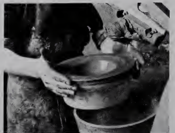
6. Take the mold out of the cuphead. Leave the finished article in the mold to dry before firing.
