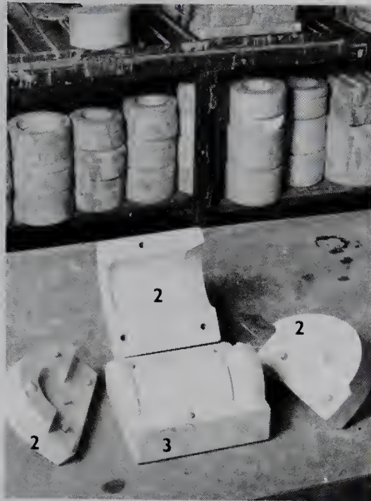
Each section of a block mold (2) is used to cast a case mold (3). Such molds are made by sealing the surface of the block molds with soft-soap solution, first thoroughly dampening the plaster. What was reversed in the block now becomes a solid relief. The two end pieces — the outer case — make it easier to pour the plaster onto the sealed case molds. The end result is a series of working molds.
