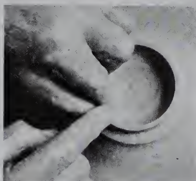
6. The final shaping of the flange is done by gently holding and supporting the wall with the left hand, while the forefinger of the right smooths the top rim.
