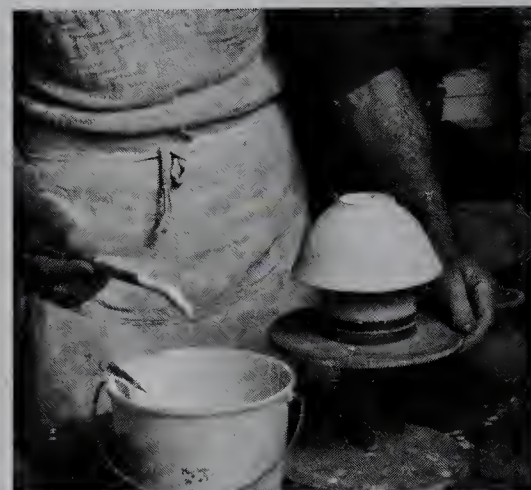
2. When using a brush it is difficult to apply the glaze evenly. Several coats of glaze should be applied.
