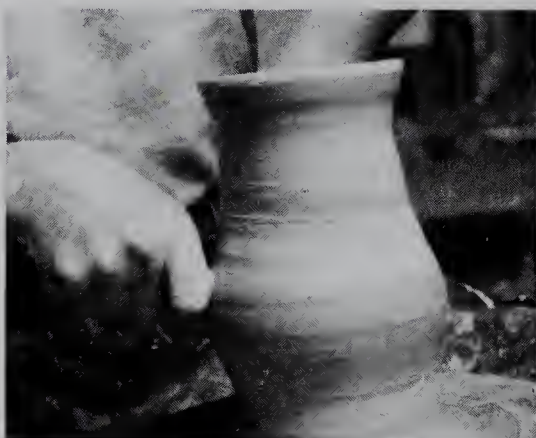
7. The vase is thinned as it begins to take shape. Pressure is applied with the flat edge of the right hand's first finger while the fingertips of the left resist this pressure, lifting the clay upwards from the bottom of the vase.
