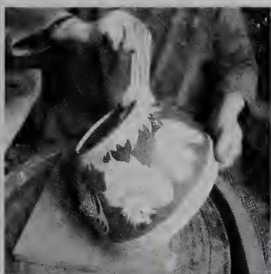
3. Clay dust and particles left at the edges of scratched lines are brushed off, otherwise they will be caught in the glaze and give a rough surface to the pot.
