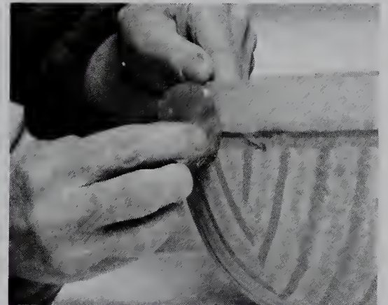
10. When the joined sections are almost leather-hard and the bowl is able to hold its shape, the pot is removed from its mold and a rim of patterned clay attached to the bowl's outside. Carefully scrape the bowl's edge with a metal kidney to smooth the surface.
