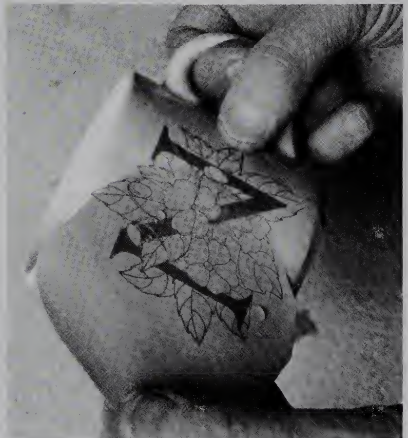
8. The transfer is soaked in water until the image begins to slide off the paper, when it is applied to the mug. Soft glue on the underside of the covercoat and
