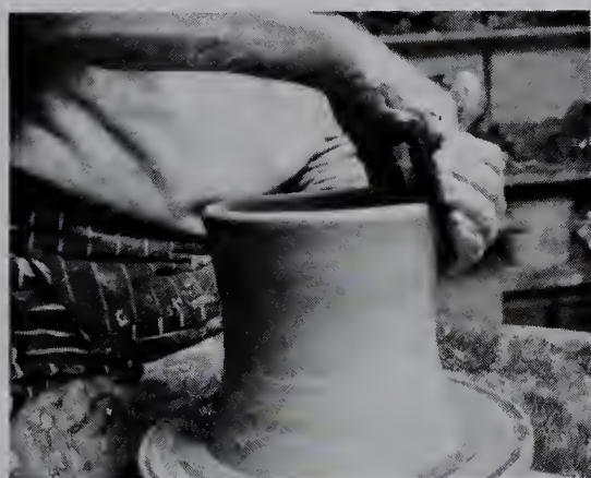
3. The hands guide the pot lightly for the final phase of lifting. The clay tends to expand outwards as it thins so that collaring will be necessary to control it after each thinning movement.
