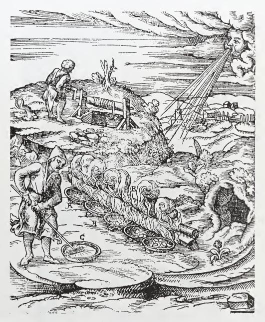
**FIGURE 14** ■ Smelting of bismuth ore in open wind; freshly formed molten bismuth flows into the pans (Ercker, see Fig. 4).
