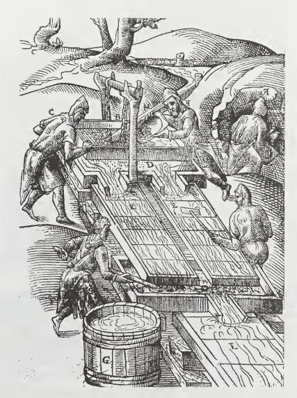
FIGURE 7 ■ A sixteenth-century machine washing alluvial gold ores (Ercker, see Fig. 4). Gold's great density (19.3 g/cm³) permits its ready separation from other, lighter minerals.
