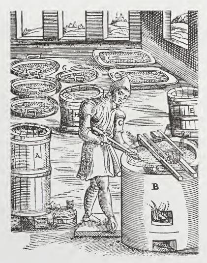
FIGURE 16 Pans and tubs from crystallizing concentrated leachate for saltpetre (see Fig. 15). One hundred pounds of the concentrate yields about 70 pounds of saltpetre (Ercker; see Fig. 4).
