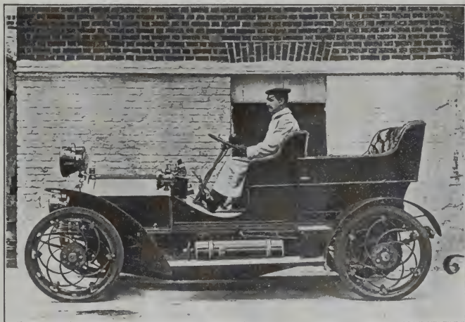
Figure 3.5.4. Car headlights with dissous gas. From Anonymous (1906).
