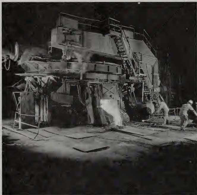
Figure 7.3.5. Oxygen lancing at the Domnarfvet steelworks, Sweden, ca. 1970. Courtesy of AGA Historical Picture Archive.
