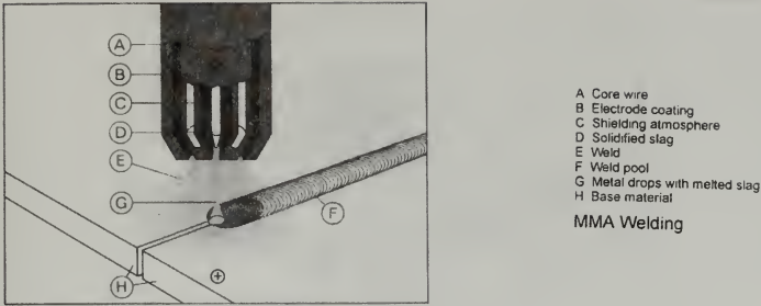
Figure 7.2.20. Arc welding with flux-coated electrode (principle). Courtesy of AvestaPolarit Welding, Avesta, Sweden.
