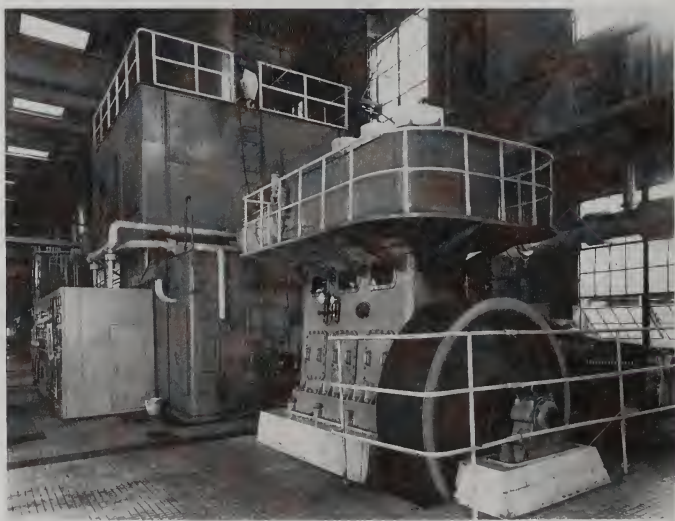
Figure 5.8.5. Interior of the first LOX plant, LOX compressor. Courtesy of Nippon Sanso Corporation, Tokyo, Japan.
