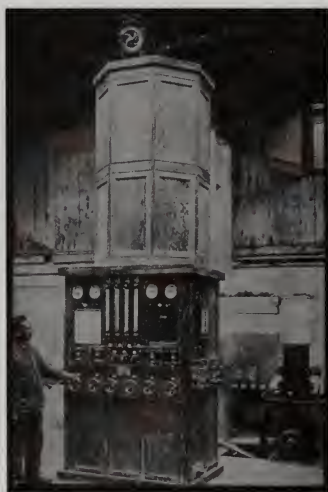
Figure 5.4.3. Operation of an early air separation column. From L'Air Liquide (1992) with permission.
