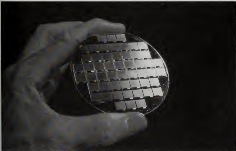
Figure 7.7.3. Semiconductor wafer. From Lockhart (1986) with permission.
