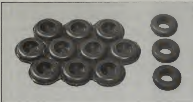
Figure 7.6.11. Rubber gaskets before and after cryogenic deflashing. Courtesy of the AGA Historical Picture Archive.
