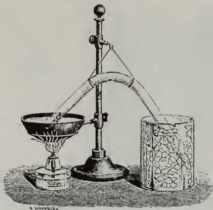
Figure 3.4.4. Faraday's equipment for the liquefaction of gases.
