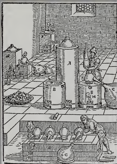
Figure 3.3.6. Nitre bed/nitric acid preparation (Lazarus Ercker, ca. 1550).
