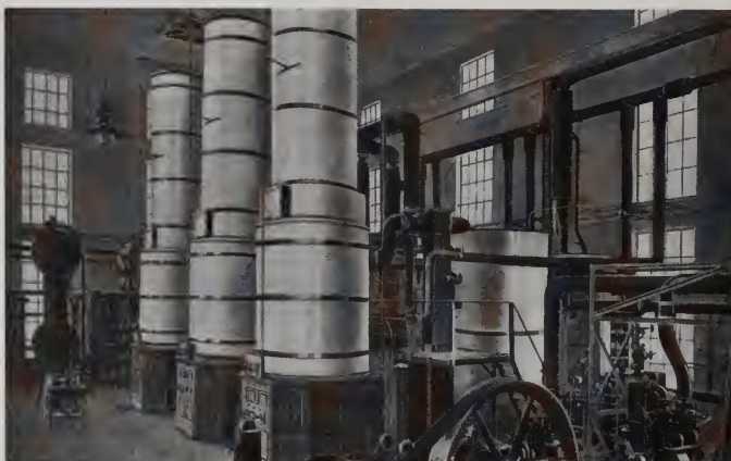
Figure 4.3.5. Early Linde plant with three units each producing 300 cubic meters of oxygen per hour. From Claude (1926).
