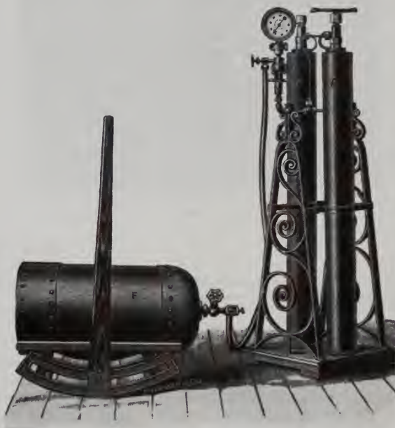
Figure 5.1.4. Liquid Carbonic developed a new "rocking" carbonator in the 1890s. From Stiegerwald (1988) with permission.
