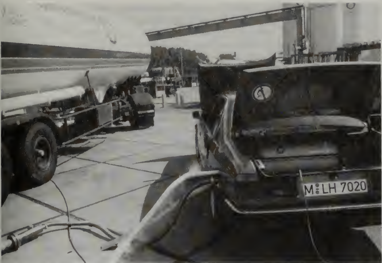
Figure 5.3.11. Messer equipment development project for using liquid hydrogen as a car fuel. From Koch (1993) with permission.
