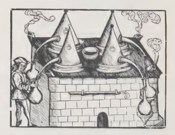
Fig. 1.7. DISTILLATION APPARATUS WITH ROSENHÜTTE. (From Brunschwygk, The vertuose Boke of Distyllacyon of the Waters of all manner of Herbes . . . [1527].)
