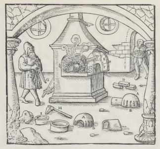
Fig. 1.13. Assay furnace and other assay equipment. (From Agricola, De re metallica [1556].)
