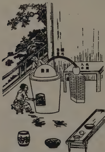
Fig. 5. Chinese still for preparing mercury. (From Li, Chemical Arts of Old China .)
