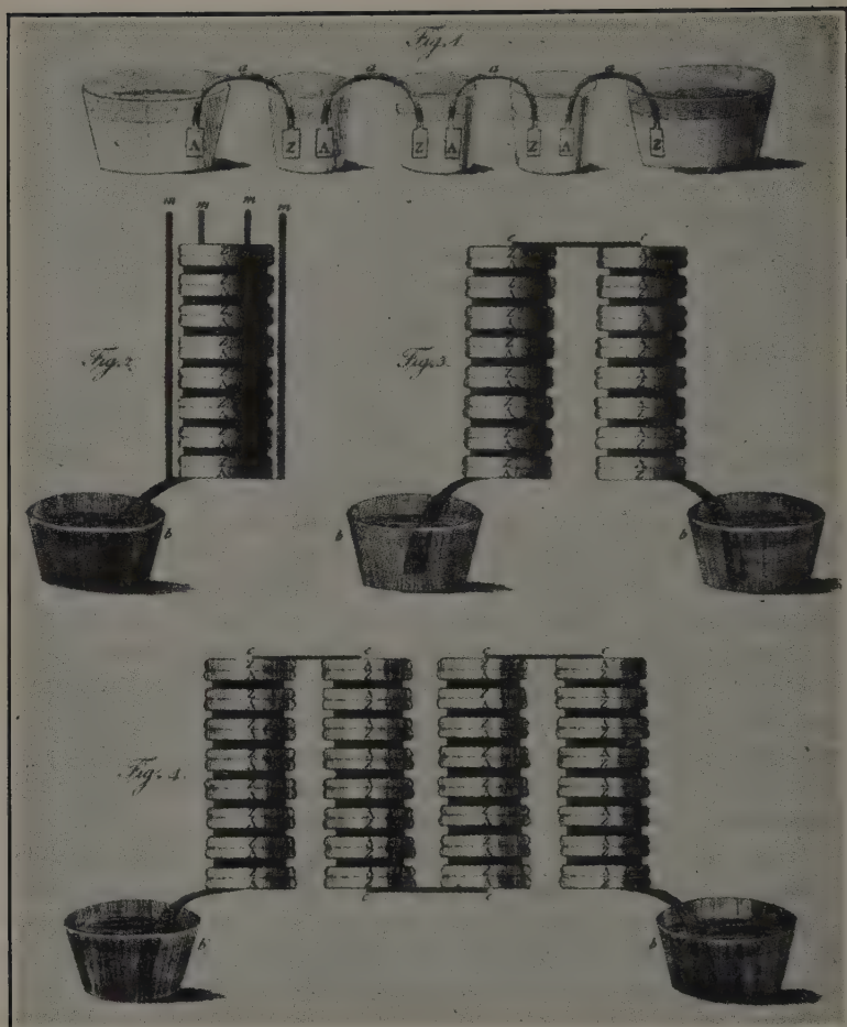
Fig. 14. Forms of the voltaic pile used by Volta. (From Philosophical Transactions of the Royal Society , 1800, p. 431.)
