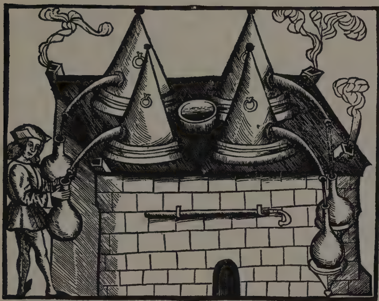
Fig. 8. Water bath and stills with Rosenhut . (From H. Brunschwygk, Liber de arte distillandi de simplicibus .)
