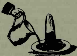
FIG. 9. Porosity of a column of salt
