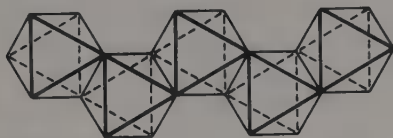
Fig. 22-A-1. The zigzag \text{ZrCl}_6 chains in \text{ZrCl}_4 .
