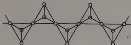
Fig. 12-3. A linear chain silicate anion.
