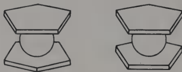
Fig. 3-12. Staggered and eclipsed configurations of an (\eta-C_5H_5)_2M compound. In crystalline ferrocene there are molecules of different orientations randomly distributed throughout the crystal (P. Seiler and J. D. Dunitz, Acta Cryst. , 1979, B35 , 1068). Also, the H-atoms of the rings are bent towards the metal (F. Takasagawa and J. F. Koetzle, Acta Cryst. , 1979, B35 , 1074).
