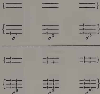
Fig. 20-18. Sketches of the unique ground state occupancy schemes for d orbitals in octahedral complexes with d configurations d^1 , d^2 , d^3 , d^8 , d^9 , d^{10} .
