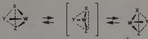
Fig. 28-14. The inversion of a pyramidal molecule WXYZ . Note that if X , Y , and Z are all different, the invertomers are enantiomorphous.
