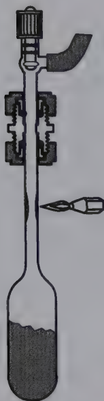
Figure 8.17 Sealing larger glass ampoules under vacuum.
