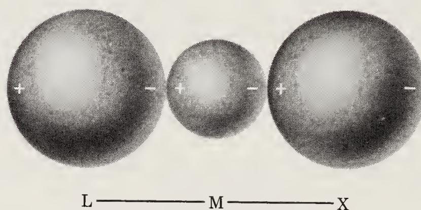
Figure 6-8 Arrangement of dipoles according to the polarization theory of the trans effect.
