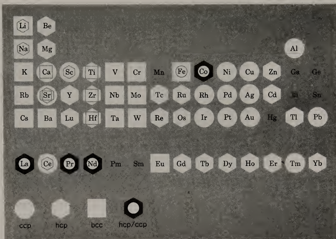
Figure 8-6 The occurrence of hexagonal close-packed (hcp), cubic close-packed (ccp), and body-centered cubic (bcc) structures among the elements. Where two or more symbols are used, the largest represents the stable form at 25°C. The symbol labeled hcp/ccp signifies a mixed . . . ABCABABCAB . . . type of close packing, with overall hexagonal symmetry. [Adapted with permission from H. Krebs, Grundzüge der Anorganischen Kristallchemie , F. Enke Verlag, 1968.]
