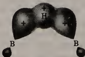
Figure 3-34 The formation of three distinct three-center molecular orbitals in a B—H—B bridge system.
