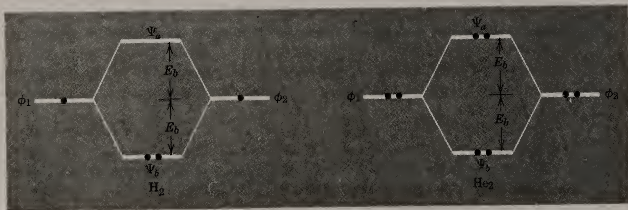
Figure 3-19 MO energy-level diagrams for the \text{H}_2 and \text{He}_2 molecules. The orbitals marked \phi_1 and \phi_2 are the contributing 1s atomic orbitals on either two H or two He atoms. The MO's marked \Psi_a and \Psi_b correspond to those diagramed in Fig. 3-17.
