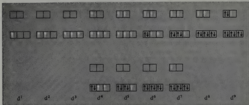
FIG. 19.14 The possible high-spin and low-spin configurations arising as a result of the imposition of an octahedral crystal field on a transition metal ion.
