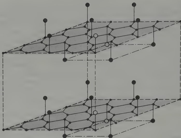
FIG. 8.7 Proposed structure for C_4F showing retention of the planar graphite sheets but with regularly spaced F atoms above and below each layer. The spacing between successive C layers is \sim 534 pm (cf. CF \sim 817 pm) and the density is 2.077 g cm ^{-3} .
