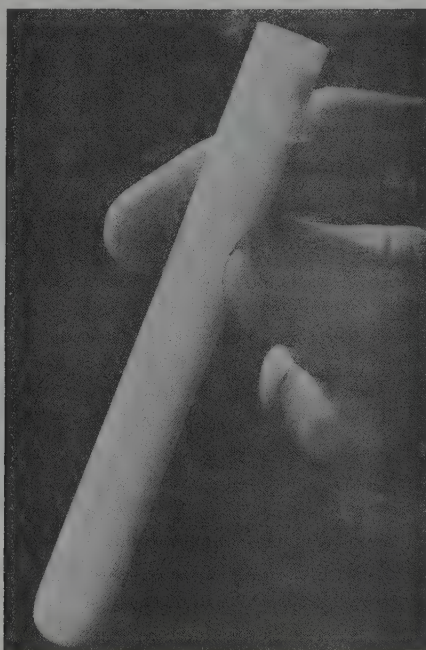
FIG. A Beta-alumina ceramic electrolyte tube. (From the Electricity Council Research Centre, Sodium Sulfur Batteries for Traction , 1974.)
