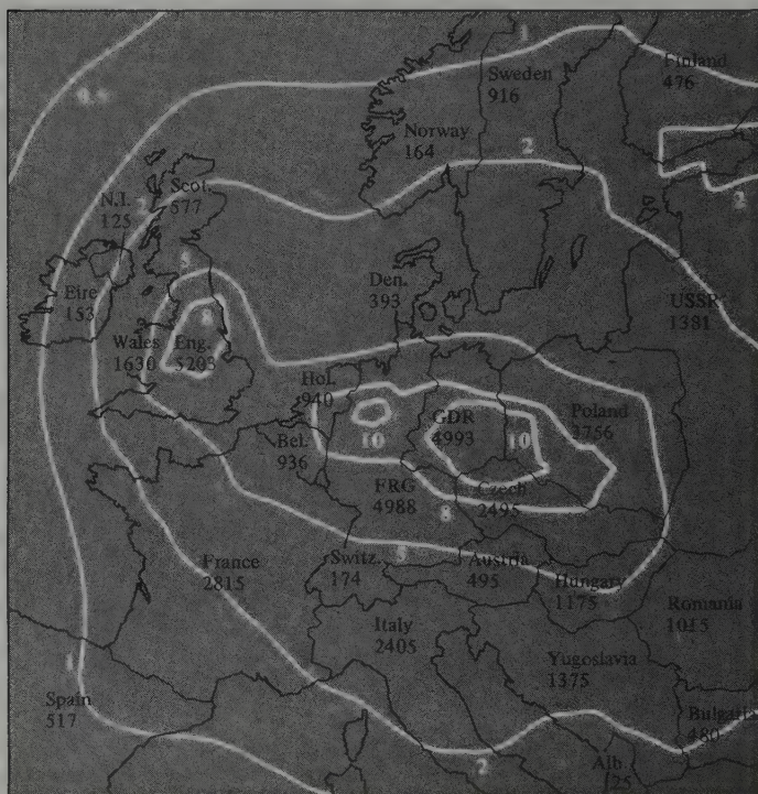
FIG. B Dry plus wet deposition of \text{SO}_2 from all the European sources shown, expressed as contour lines in \text{g}(\text{SO}_2) \text{m}^{-2} \text{y}^{-1} . The emission strengths for each country are shown in units of 10^3 tonnes of \text{SO}_2 per year. (98f)
