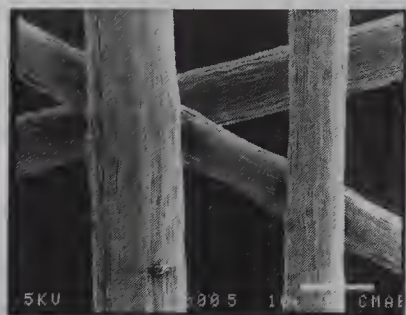
Figure 2 SEM image of boron nitride fibres obtained from (3)
