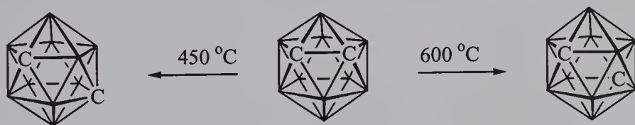
Figure 1 Isomerisation of C_2B_{10}H_{12}
