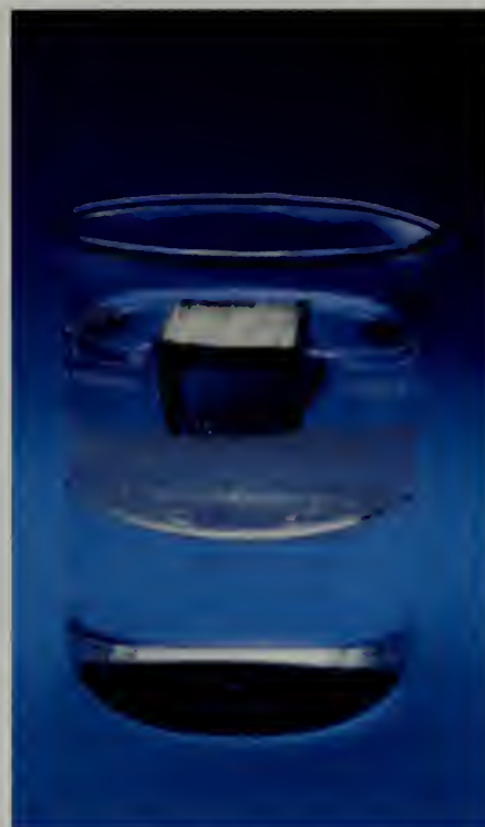
Lithium floating on a layer of oil, which is less dense than water. Lithium is the least dense of metals. (Source: Chip Clark)
