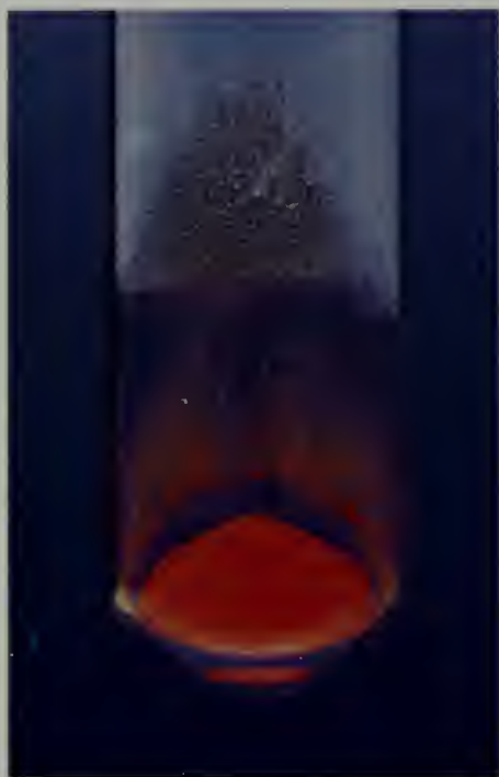
Heating red mercury(II) oxide causes it to decompose to mercury and dioxygen. The metallic mercury condenses on the cooler upper walls of the tube. (Source: Chip Clark)
