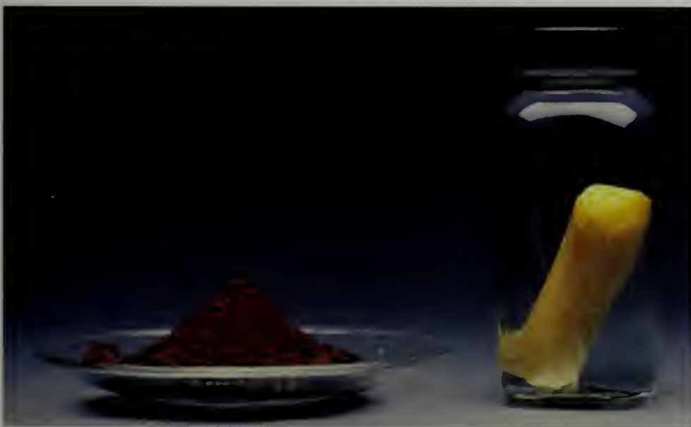
White phosphorus and red phosphorus. These two common allotropes of phosphorus differ considerably in physical and chemical properties. For example, red phosphorus is air-stable, whereas white phosphorus burns in contact with the air. Hence the white allotrope is stored under water. (Source: Chip Clark)
