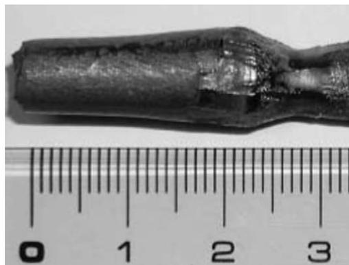
**FIGURE 8** A photograph of a floating zone (FZ) grown  $\text{TmB}_{44}\text{Si}_2$  crystal (Mori, 2006a). The scale is in centimeters.
