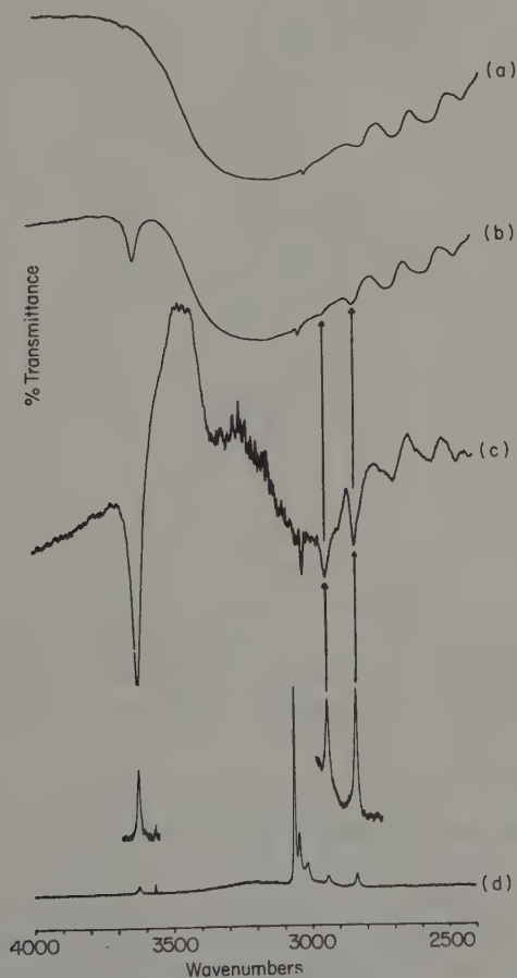
Fig. 7. Infrared spectra of (a) \beta -quinol/KBr disc (b) \beta -quinol/ \text{CH}_3\text{OH} /HCBD mull/CsI plates (c) Expanded difference spectrum, difference factor = 0.66 (d) Raman spectrum of \beta -quinol/ \text{CH}_3\text{OH} clathrate.
