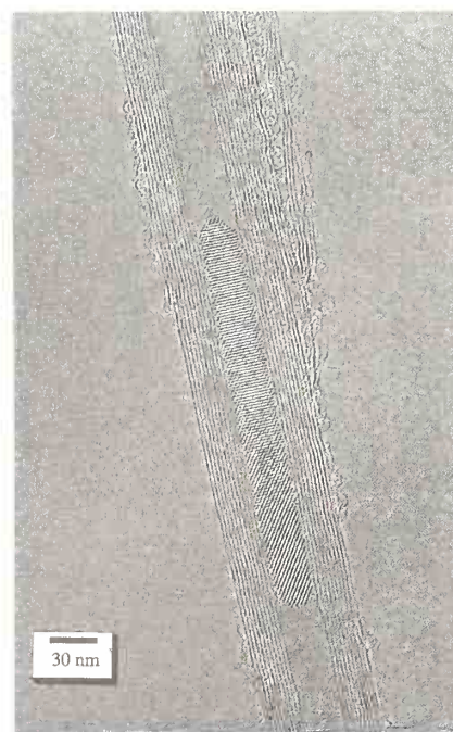
10.22 Electron micrograph of samarium(III) oxide inside a carbon nanotube. (J. Cook, J. Sloan, and M.L.H. Green, Chem. in Industry , 600 (1996).)
