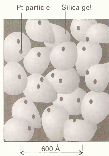
17.5 Schematic diagram of metal particles supported on silica gel.
