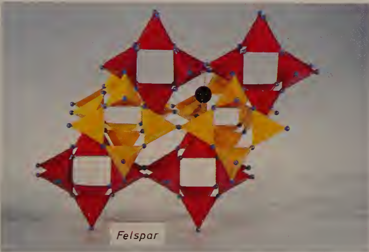
Figure XV.24. Model of the feldspar structure with regular tetrahedra viewed along b .
