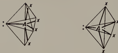
Figure 3. (a) Gillespie's model, illustrating the deviations from the ideal shapes of AX_4E molecules. The lone pair forms a corner, while the cation forms the center of a polyhedron. (b) Our model. The lone pair-X distance is determined from the ideal trigonal bipyramid. Angles and distances are simply a function of atom sizes. The lone pair plus attached cation form a corner of the polyhedron, the center of which is empty.
