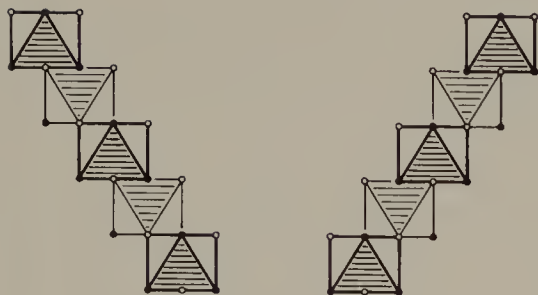
Figure 22. The diagonal string of corner-sharing octahedra common to the corundum, rutile, B-Nb 2 O 5 , and PdF 3 structures: two alternative equivalent orientations. [Corner-connected across the mirror plane, these units also appear in the structures of Fe 3 C etc. (below).]
