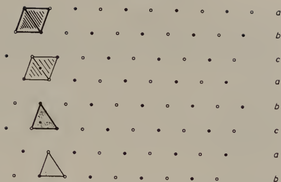
Figure 1. Cubic close packing, ccp. Smaller circles are at the centers of the polyhedra. All atoms are on 0 or \frac{1}{2} .
