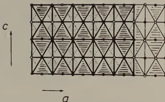
Figure 5. The idealized structure of NiAs.
