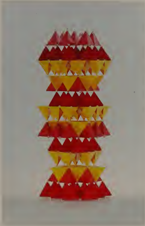
Figure VII.2. A model of the \text{Al}_4\text{C}_3 structure: Al atoms in \text{C}_4 tetrahedra.
