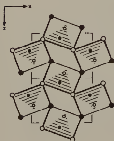
Figure 24. FeB projected on (010). Large circles are Fe; small circles are B; open at y = \frac{1}{4} , filled at y = \frac{3}{4} . (Compare with Figure 28 of Chapter IV.)
