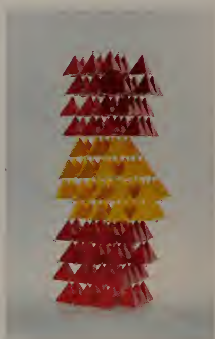
Figure VII.1. (b) A model of 8H-SiC.
