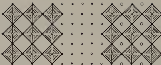
Figure 20. The structures of \text{ReO}_3 (left) and \text{SrTiO}_3 . Complete ccp is shown in the center.
