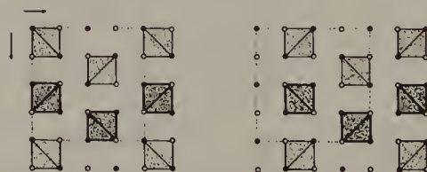
Figure 15. The idealized (but very close to the real) structure of SnI_4 (as two bounded projections).
