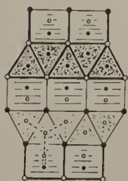
Figure 19. The \alpha -ThSi 2 structure projected on (010); all atoms are at 0 or \frac{1}{2} . Compare with Figure 18, from which structure this one is readily derived by CS, and also Figure 1. (The broken lines indicate part of the three-dimensional, 3-connected silicon net.)
