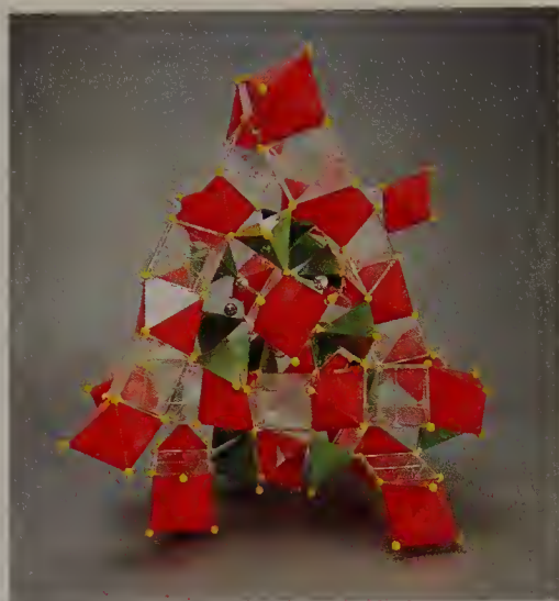
Figure XV.3. Polyhedral model of garnet. Note the rods of alternating octahedra and trigonal prisms sharing faces. Such rods pack as in Figure 2 of Chapter XV.
