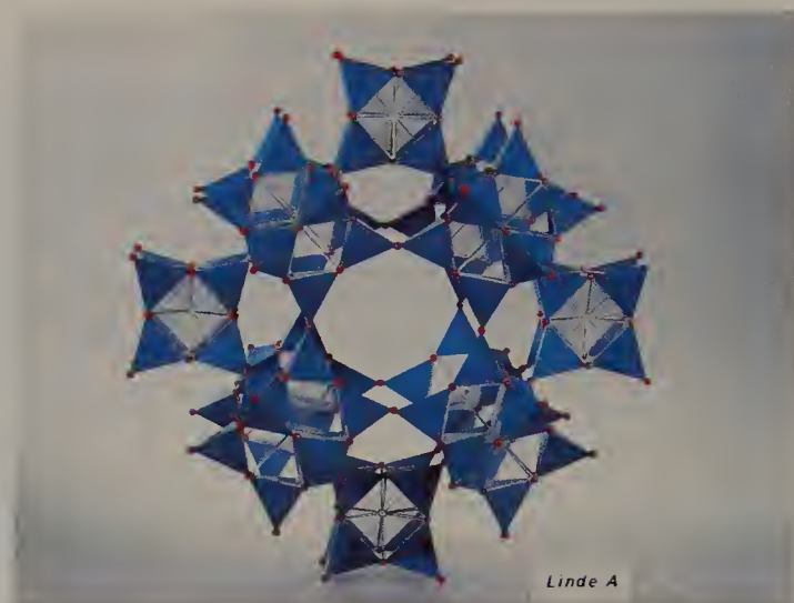
Figure XV.29. Polyhedral model of Linde A.
