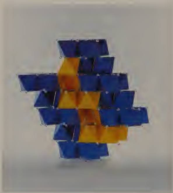
Figure IV.15. Octahedral model of \text{Al}_2\text{O}_3 . Blue and yellow parts are rutile.
