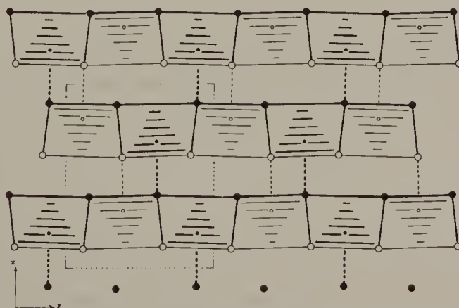
Figure 21. \text{SrBr}_2 \cdot \text{H}_2\text{O} projected on (010) of Pnma . Small circles are Sr; large circles are Br; open at y = \frac{1}{4} , filled at y = \frac{3}{4} . ( \text{H}_2\text{O} molecules are not shown.) Dotted lines are bonds from Sr to the Br atoms capping the \text{SrBr}_6 trigonal prisms.
