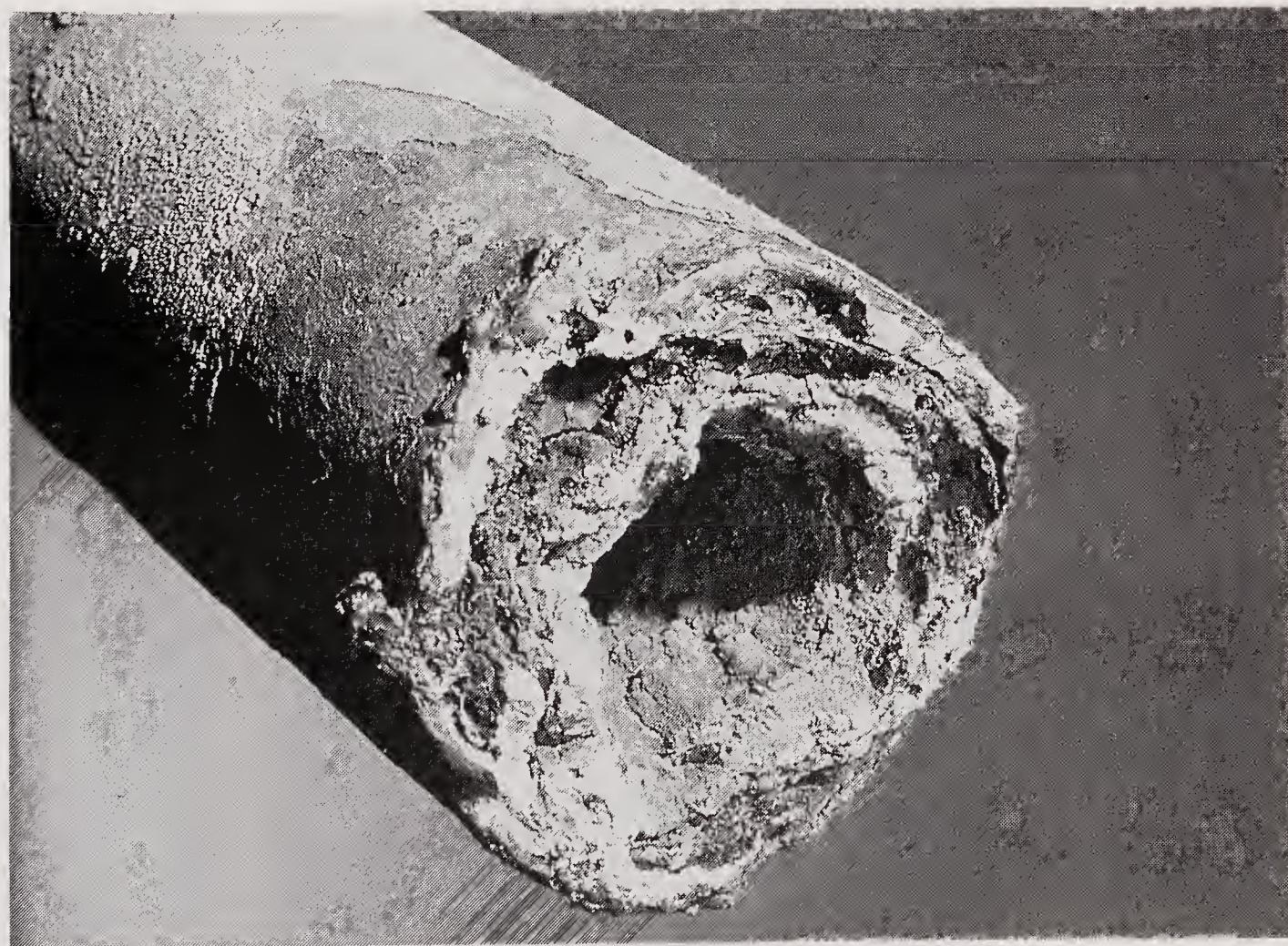
FIGURE 13.8 A hot water pipe filled with a predominantly \text{CaCO}_3 deposit. (Betz Industrial.)
