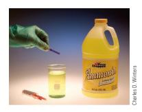
Figure 17-8 Ammonia-based cleaning solution. Ammonia solution turns red litmus paper blue, indicating that ammonia is a base, removing protons from a small fraction of the water molecules to yield a low but detectable concentration of hydroxide ions.
