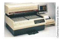
Figure 20-6 Scintillation counter. This instrument is especially useful for detecting gamma radiation because it uses a high-density transparent solid, in contrast with the low-density gas in a Geiger counter. Radiation interacts with the solid, resulting in flashes of light, which are counted by a detector.
