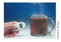
Figure 3-24 An infrared thermometer. When conventional temperature sensors cannot be used, a noncontact device such as this infrared thermometer is used instead. A lens focuses the infrared light emitted from a heated object onto a detector, which is calibrated to convert the wavelength of light to an electronic signal that can be displayed as temperature.
