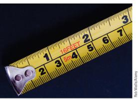
Figure 3-8 Length measurements: inches, centimeters, and millimeters. This illustration is very close to full scale. The numbers and the long lines on the top scale are inches, and the numbers and the long lines on the bottom scale are centimeters. One inch is defined as 2.54 centimeters, which is the same as 25.4 millimeters (shorter unnumbered lines).
