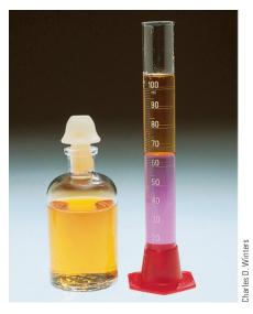
When an aqueous bromine solution (*orange*) is added to a solution containing iodide ion, bromide ion and iodine (*purple*) are formed. Two different solvents are used to separate the products.
