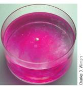
Sodium metal reacts with water, forming sodium ion, hydroxide ion, and hydrogen gas. A compound that changes from colorless to pink when it reacts with hydroxide ion was added to the water before the sodium.
