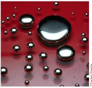
Mercury drops. Notice that the larger the drop, the greater the degree to which it is flattened by the force of gravity.
