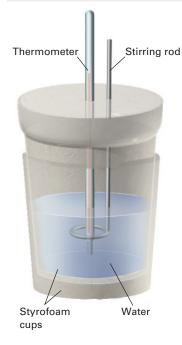
Figure 15-41 Coffee-cup calorimeter. Data for heat-flow problems are obtained from calorimeters, highly insulated containers in which chemical or physical changes occur. This coffee-cup calorimeter is commonly used in introductory college chemistry laboratories.
