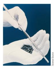
Figure 20-25 Nuclear fuel. After mining, uranium is usually enriched to  $3.5\%_{92}^{235}U$  in the form of uranium oxide, UO2, powder. The powder is pressed into pellets, which are then inserted into tubes called fuel rods.
