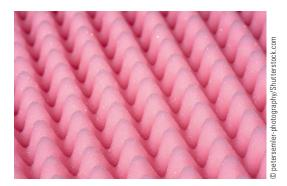
Aniline is used in the polyurethane manufacturing process. Materials made from polyurethane include foams (as pictured), spandex, hardwood floor coatings, dolly wheels, and many other end products.
