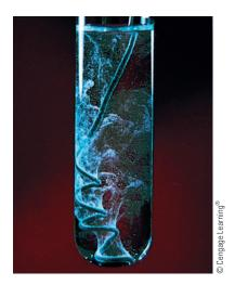
Aluminum metal reacts with hydrochloric acid, releasing bubbles of hydrogen gas.
