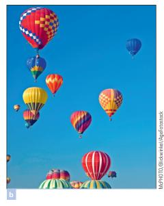
Figure 14-12 Gas density and floating balloons. (a) A helium-filled balloon floats, but air-filled balloons lie on the surface of the table. The density of helium is lower than that of air at the same temperature and pressure. (b) Hot air balloons float because the higher temperature of the air enclosed in the balloon makes it less dense than the surrounding air.
