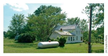
**Figure 9-12** Rural homes that do not have access to natural gas pipelines can use liquid propane as a source of fuel for their furnaces and hot water heaters. The propane is stored in large tanks that are refilled periodically.
