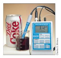
Figure 18-23 Measuring the pH of cola. Note that the solution is quite acidic. Nonetheless, the weak acid in the solution is only slightly ionized.
