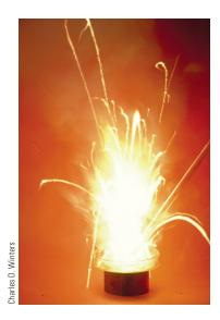
Figure 19-14 The reaction between iron(III) oxide and aluminum releases so much energy that *liquid* iron is formed as one of the products. Iron(III) oxide is the oxidizing agent, and aluminum is the reducing agent.
