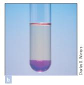
Figure 19-4 Preparation of bromine. (a) Chlorine gas is bubbled through a solution of sodium bromide. (b) The liquid bromine product is extracted by adding carbon tetrachloride. The top water layer and the bottom carbon tetrachloride layer both contain dissolved bromine, but it is more concentrated in the bottom.
