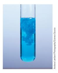
Copper(II) hydroxide precipitates.
