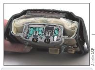
When a car decelerates in a collision, an electrical contact is made in the sensor unit. The propellant (green solid) detonates, releasing nitrogen gas, and the folded nylon bag explodes out of the plastic housing.
