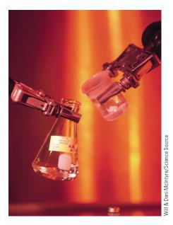
Remotely operated robotic arms are used to maneuver dangerously radioactive samples.
