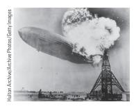
Figure 8-11 The end of the Hindenburg dirigible in May 1937. The explosion demonstrates the tremendous amount of energy released when hydrogen reacts with oxygen to form water. This disaster ended the use of hydrogen in lighter-thanair aircraft. Today, the unreactive Group 8A/18 gas, helium, is used in blimp airships—from which aerial views of major sporting events are displayed on television.
