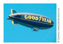
Figure 11-37 An airship. The "lighter than air" feature of an airship comes from the low-density helium that fills it. Helium is safe for this purpose because it is unreactive, unlike even lower density hydrogen. See Figure 8-13.
