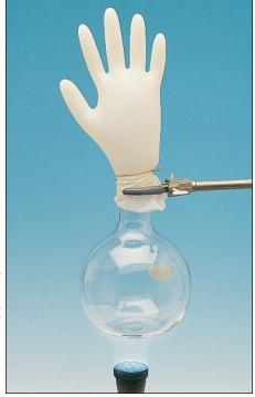
Figure 4-17 Volume and temperature of a gas. For a fixed amount of a gas at constant pressure, the volume and the Kelvin temperature of the gas are directly proportional to each other. As the temperature increases, the volume increases proportionally.
