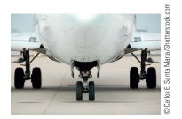
Figure 14-10 The Federal Aviation Administration requires that the tires of large commercial jet aircraft be filled with nitrogen because it will not support combustion if a tire fire occurs.
