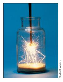
**Figure 18-9** The glowing splint test for oxygen.
