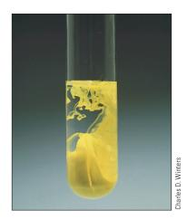
**Figure 16-27** Solid lead(II) iodide precipitates.
