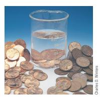
**Figure 19-18** Metallic copper does not react with a strong acid to release hydrogen because copper and hydrogen ion are weaker reducing and oxidizing agents than hydrogen gas and copper ion, respectively.
