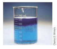
Ammonia solution (colorless) was added to a solution of hydrated copper(II) ions (light blue, *bottom*), yielding  $Cu(NH_3)_4^{2+}$ (aq) (dark blue, *top*).
