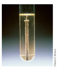
**Figure 19-3** Iron metal is added to a hydrochloric acid solution. Hydrogen gas is bubbling from the solution.
