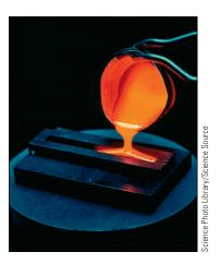
Figure 20-29 Vitrification is one technique for storing nuclear waste. The liquid waste is heated to a high temperature and mixed with substances that form a glassy solid when cooled. This prevents problems associated with storing liquids in tanks that may leak.
