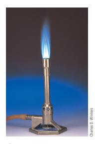
Figure 21-17 Combustion of natural gas. Hydrocarbons, such as natural gas, burn in air, releasing a relatively large amount of energy. This energy is then used to generate electricity; operate engines; heat factories, businesses, and homes; and, in general, to provide energy for most of the conveniences of modern society.
