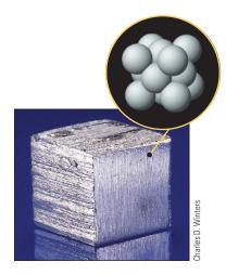
**Figure 15-37** Aluminum metal. This is an example of a metallic crystal.
