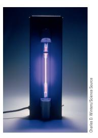
**Figure 14-9** An argon-gas-filled discharge tube, emitting the blue glow characteristic of argon.
