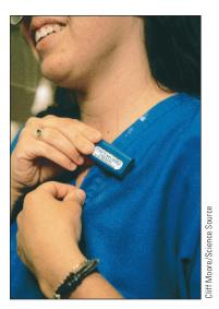
**Figure 20-8** Film badge. Workers in industries in which exposure to radiation is known to be above background levels are required to monitor their cumulative exposure dosage.
