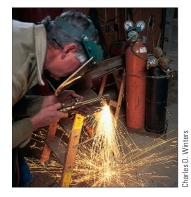
Figure 21-11 Oxyacetylene torch. Acetylene is the fuel in a welder's torch. It reacts with the oxygen in the air in a highly exothermic reaction, producing a 3000°C flame, which is hot enough to cut through
