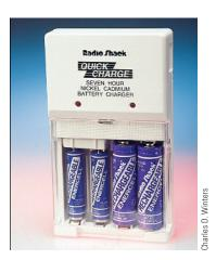
**Figure 19-7** Nickel-cadmium (ni-cad) batteries. The fundamental components of these batteries are nickel oxide, nickel hydroxide, and nickel metal, cadmium hydroxide and cadmium metal, and potassium hydroxide.
