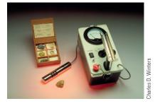
A Geiger-Müller counter is used to detect ionizing radiation.
