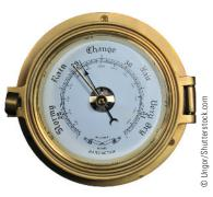
Figure 4-9 A mechanical gauge used to measure atmospheric pressure. In general, mechanical gauges work via an air-filled tube that changes shape with changing pressure. Levers and/or gears move in response to the tube, and a pointing needle and scale or an electronic display is calibrated to show the corresponding atmospheric pressure.
