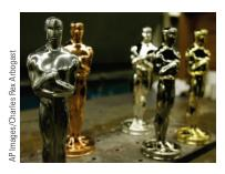
Figure 19-11 Electroplating. An electrolytic cell is used to add a coating of a relatively expensive metal to a less expensive base metal. The base metal for the Oscar statues shown here is brittanium, an alloy (solid solution) of tin, copper, and antimony. They are then sequentially electroplated with copper, nickel, silver, and, finally, 24-karat gold.
