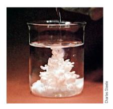
Silver nitrate solution is added to an unknown chloride-ion solution, yielding a precipitate of silver chloride.
