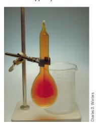
Nitrogen monoxide and oxygen, both colorless gases, react to form reddish-brown nitrogen dioxide.
