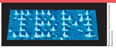
**Figure 11-25** Arrangement of xenon atoms to spell IBM. The logo is composed of 35 xenon (Z = 54) atoms, *individually* moved using a scanning tunneling microscope. The space between the atoms is about 1.3  $\times$  10<sup>-7</sup> cm. As printed, the magnification is 4.7 million.
