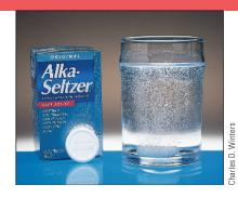
**Figure 17-19** Alka-Seltzer®. The solid tablets contain both citric acid and sodium hydrogen carbonate, which cannot react until they are dissolved in solution. Once dissolved, an acid-base reaction takes place, forming bubbles of gaseous carbon dioxide.
