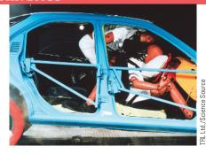
**Figure 14-17** The crash test dummy in the driver's seat is restrained by a seat belt and an inflated air bag. The dummy in the back seat, not wearing a seat belt, is being propelled through the cabin toward the front windshield.
