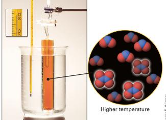
equilibrium is shifted in the forward direction. The concentration of  $N_2O_4$  molecules is relatively high. At higher temperature (right tube) the gas is much darker because brown  $NO_2$  is formed as the reaction shifts in the reverse direction. The  $N_2O_4$  concentration has decreased.
