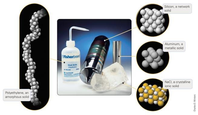
**Figure 15-25** Amorphous (*left*) and crystalline (*right*) solids. An amorphous solid, such as the polyethylene bottle shown, has little long-range ordering at the particulate level. In contrast, each of the crystalline solids shown has an orderly, regularly repeating arrangement of the particles.
