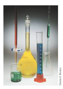
Figure 3-13 Volumetric glass-ware. The beaker is only for estimating volumes. The tall graduated cylinder is used to measure volume more accurately. The flask with the tall neck (volumetric flask) and the pipet are used to obtain samples of fixed but precisely measured volumes. The buret is used to dispense variable volumes with high precision.
