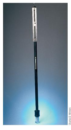
A mercury-free barometer is often used in introductory chemistry laboratories.
