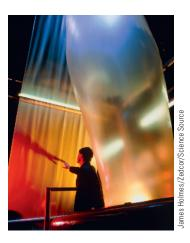
**Figure 21-41** Polyethylene film. Sheets are manufactured by squeezing the liquid through a thin opening and inflating it with air.
