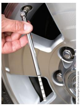
**Figure 4-10** Tire pressure gauge. Most tire pressure gauges have a piston inside the casing that is attached to a spring. A plastic rod rides on top of the piston. When the gauge is placed on a tire valve stem, the air in the tire pushes on the piston, which pushes the calibrated rod out. When the gauge is removed, the spring pushes the piston back, but the rod remains in the same position to allow you to read the tire pressure.
