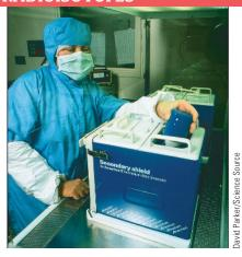
**Figure 20-22** Radioisotope generator. The most widely used radioisotope generator converts molybdenum-99 to technetium-99m, in which the *m* indicates that the isotope is *m*etastable, which means that the nucleus is in a temporary high-energy state. The excess energy is given off in the form of gamma radiation, which is used for diagnostic procedures.
