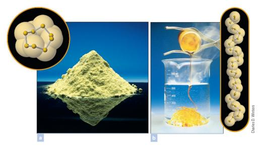
**Figure 15-30** Two forms of sulfur. (a) One form of solid sulfur is an example of a molecular crystal in which distinct molecular units can be identified. (b) One liquid form consists of chains of sulfur atoms.
