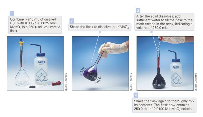
Figure 16-19 Preparing a solution of specified molarity.
