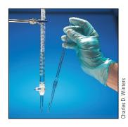
**Figure 3-19** A buret and a pipet. The buret on the left is used to deliver variable volumes to an accuracy of  $\pm 0.05$  mL. The pipet on the right is used to dispense a fixed volume of liquid with an accuracy of  $\pm 0.03$  mL. These instruments are common in introductory chemistry laboratories, but most research labs use automated titrators and automatic pipets.
