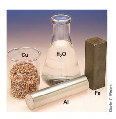
**Figure 15-39** Specific heats of water and three metals. The specific heat of liquid water, 4.18 J/g · °C, is much higher than that of the solid metals shown in this photograph: copper, 0.38 J/g · °C, aluminum, 0.90 J/g · °C, and iron, 0.45 J/g · °C. When the amount units are changed from grams to moles, you can see that the metals have very similar capacities to retain heat energy on a per mole basis: copper, 24 J/mol · °C, aluminum, 24 J/mol · °C, and iron, 25 J/mol · °C.
