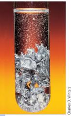
Zinc reacts with hydrochloric acid to produce zinc chloride and hydrogen gas.
