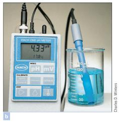
**Figure 17-15** Measurement of pH. (a) The color imparted to papers impregnated with certain dyes can be used for approximate measurements of pH. (b) A pH meter is a voltmeter calibrated to measure pH.
