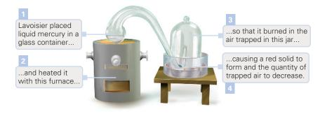
**Figure 1-4** Lavoisier's apparatus for investigating the reaction of mercury and oxygen, as illustrated in his book *Traité Élémentaire de Chime*.
