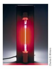
When neon gas is within an activated gas discharge tube, reddish-orange light is emitted.
