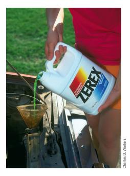
Ethylene glycol, HO–CH<sub>2</sub>–CH<sub>2</sub>–OH, is the most widely used automotive antifreeze.
