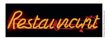
Figure 14-8 Helium-gas-filled sign. When a glass tube is filled with helium at low pressure and a high voltage is applied, current will flow and the ionizing gas will glow, producing a color characteristic of the element. Helium-filled gas discharge tubes emit a yellow glow.
