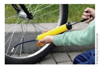
**Figure 4-18** Bicycle tire pump. When the handle is pulled up, a valve located near the point where the hose connects to the cylinder closes, and air is drawn into the cylinder. When the handle is pushed down, the valve opens, and the volume of the pump-hose-tire system decreases, causing an increase in the pressure of the enclosed gas (which is air).
