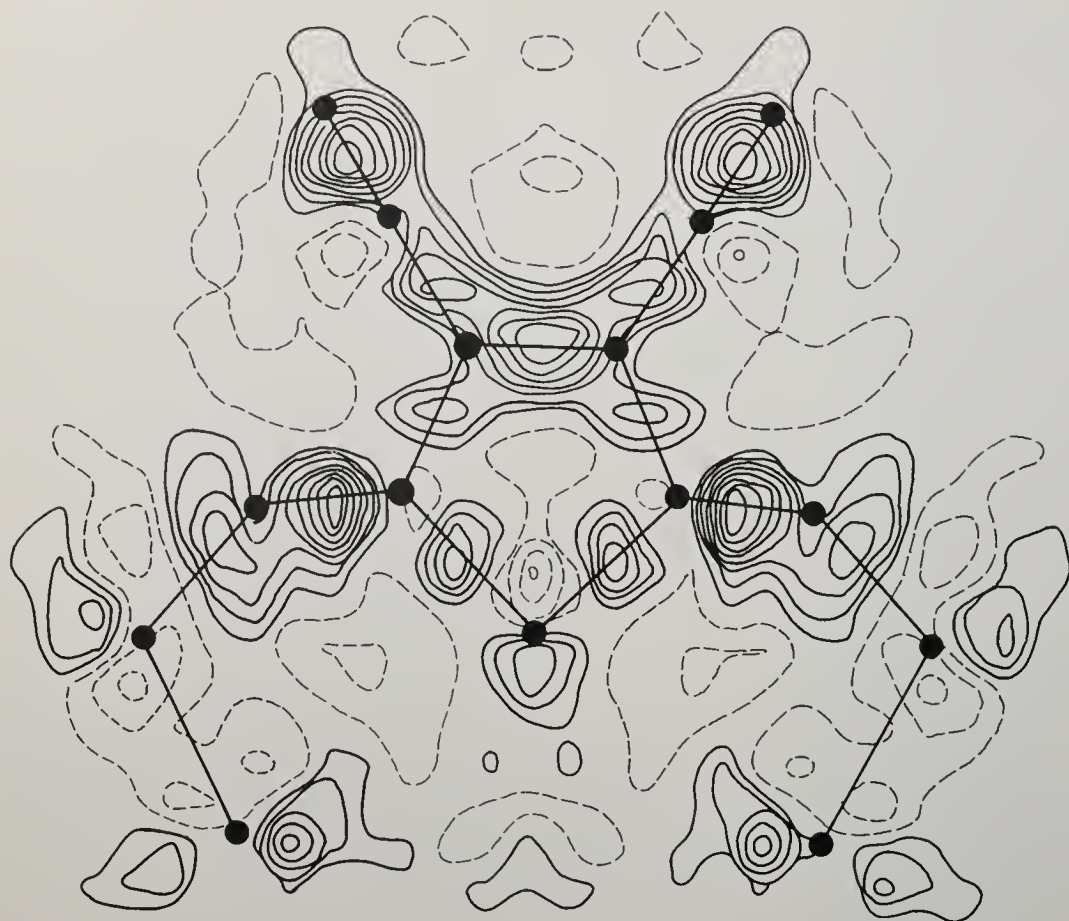
Figure 4.13 Electron density difference plot for 2,5-di- N -chlorothioimino-3,4-dicyanothiophene, obtained from x-ray diffraction data. Solid lines denote increased electron density. ( Reproduced with permission from Molecular Structure Corporation, College Station, Texas. )
