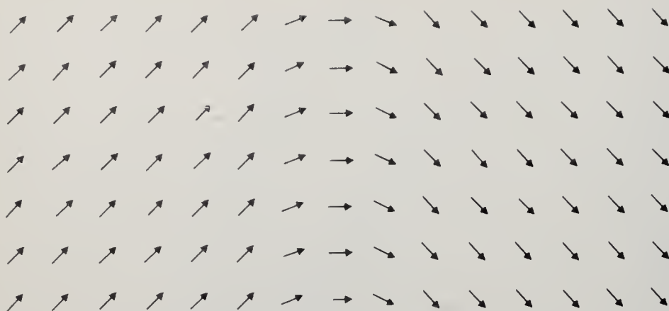
Figure 12.15 Schematic diagram of the boundary between two magnetic domains. Actual boundaries are hundreds of atoms thick. By the gradual turning of the spins within the boundary, the boundary can move in response to an applied magnetic field.
