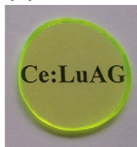
FIGURE 2.5 \text{LuAG}:\text{Ce}^{3+} single crystal grown along the \langle 111 \rangle direction by the Cz method. (a) The as-grown crystal boule, (b) the polished crystal wafer with the size of 1.0\text{ mm} in thickness [17]. Reprinted from Journal of Rare Earths , 25 (2007), Zhong Jiuping, Liang Hongbin, Su Qiang, Zhang Guobin, Dorenbos Pieter, Bir-owosuto Muhammad Danang, Effects of Annealing Treatments on Luminescence and Scintillation Properties of \text{Ce}:\text{Lu}_3\text{Al}_5\text{O}_{12} Crystal Grown by Czochralski Method , page 568, Copyright (2007), with permission from Elsevier.
