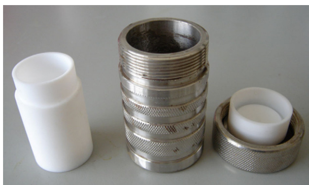
FIGURE 4.16 General purpose autoclave popularly used for hydrothermal or solvothermal synthesis.
