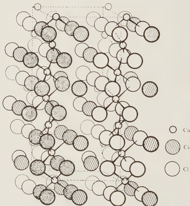
FIG. 4.32. The crystal structure of \text{CsCuCl}_3 .
