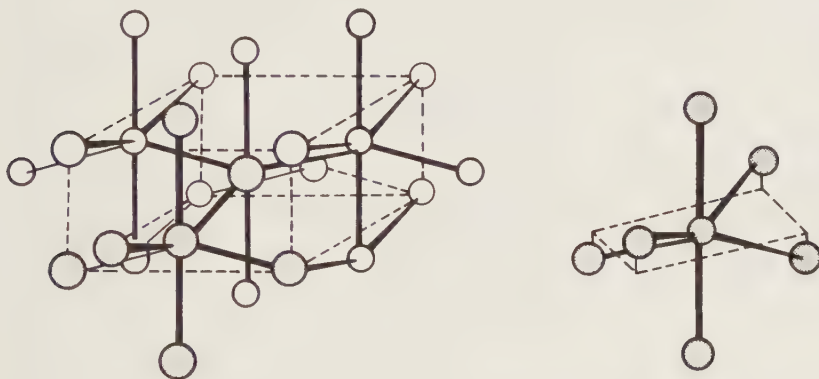
FIG. 29.2. The crystal structure of white tin, showing the deformed octahedral group of neighbours around each atom.
