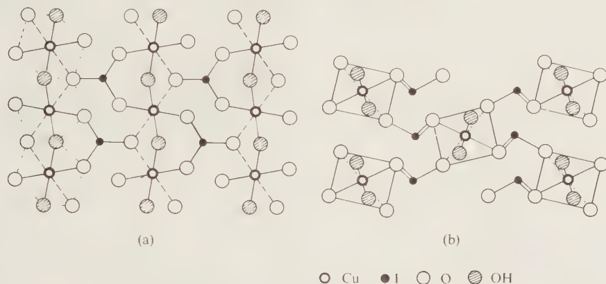
FIG. 14.16. The structure of \text{Cu}(\text{OH})\text{IO}_3 : (a) plan, (b) elevation, in which the octahedral chains are perpendicular to the plane of the paper.
