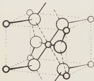
FIG. 6.6. Distorted rutile structure of \text{CuF}_2 .
