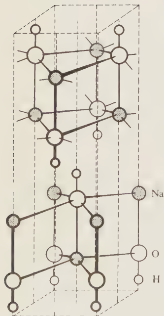
FIG. 14.4. The (yellow) TII structure of low-temperature \text{NaOH} . Since the coordinates of the H atoms have not been determined O-H has been made equal to 1 \text{ \AA} .
