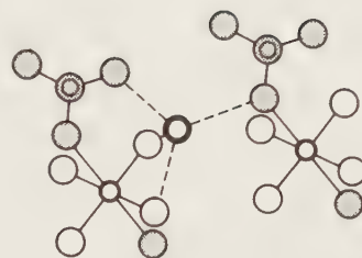
FIG. 15.15. The environment of the fifth H 2 O molecule (centre) in CuSO 4 · 5 H 2 O. The octahedral coordination group around a copper atom is composed of four H 2 O molecules and two oxygen atoms of SO 4 2- ions (shaded circles).
