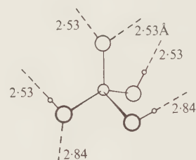
FIG. 8.12. The hydrogen bonds in crystalline \text{H}_3\text{PO}_4 .
