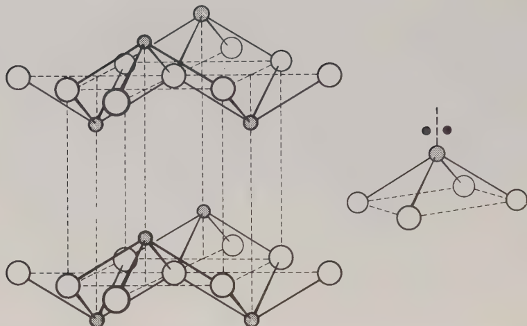
FIG. 12.14. The crystal structure of tetragonal PbO (and SnO). The small shaded circles represent metal atoms. The arrangement of bonds from a metal atom is shown at the right, where the two dots represent the 'inert pair' of electrons (see p. 1149).
