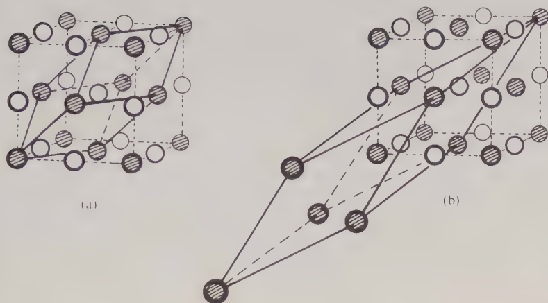
FIG. 6.3. Alternative rhombohedral unit cells in the NaCl structure.
