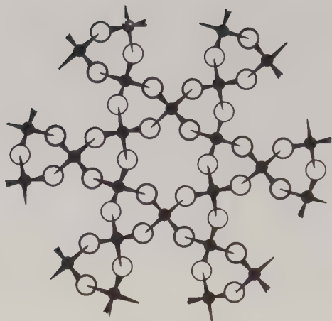
FIG. 23.6. Plan of the structure of \beta -quartz. Small black circles represent Si atoms. The oxygen atoms lie at different heights above the plane of the paper, those nearest the reader being drawn with heaviest lines. Each atom is repeated at a certain distance above (and below) the plane of the paper along the normal to that plane so that the \text{Si}_3\text{O}_3 rings in the plan represent helical chains.
