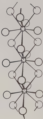
FIG. 15.14 Portion of the infinite 1-dimensional cation-water complex in crystalline \text{SrCl}_2 \cdot 6\text{H}_2\text{O} , in which each \text{Sr}^{2+} ion (small circle) is surrounded by nine water molecules.
