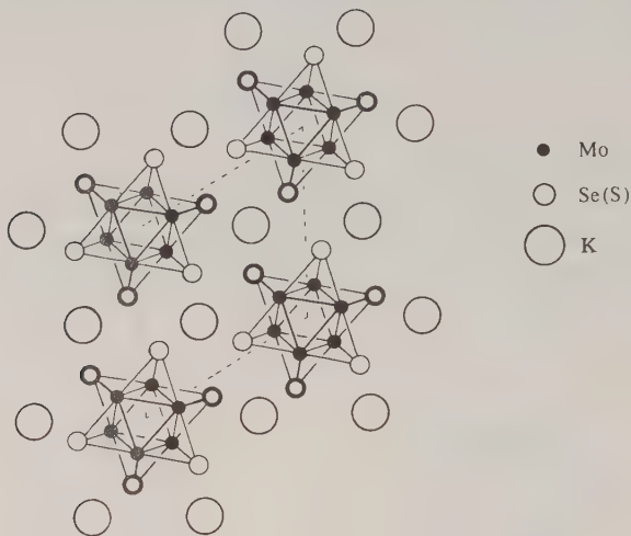
FIG. 17.19. Projection of the structure of \text{K}_2\text{Mo}_6\text{S}_6 along the chain direction.
