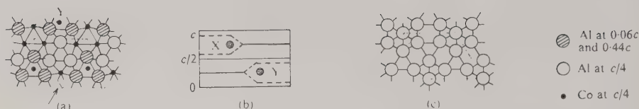
FIG. 29.18. The structure of \text{Co}_2\text{Al}_5 : (a) projection along c -axis of atoms at height \approx \frac{1}{4} , (b) elevation of one unit cell viewed in direction of arrow in (a) - X and Y are atoms which split such planes into two, (c) projection as in (a) showing atoms at height \approx 0 .
