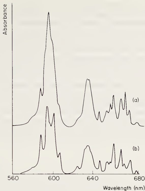
Figure 11.5 The effect of hydrogen bonding on the absorption spectrum of [\text{UCl}_6]^{2-} (a) (\text{Et}_4\text{N})_2\text{UCl}_6 in HCl-saturated \text{CH}_3\text{CN} ; (b) (\text{Et}_4\text{N})_2\text{UCl}_6 in \text{CH}_3\text{CN} (redrawn from J.L. Ryan, Inorg. Chem. , 3 (1964) 211)
