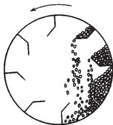
FIG. 12-27 Moving solids bed in a rotary dryer with lifters.
