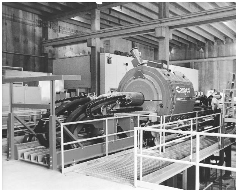
FIG. 19-54 Superconducting magnetic separator operating in a kaolin treatment plant. (Courtesy Carpco, Inc.)
