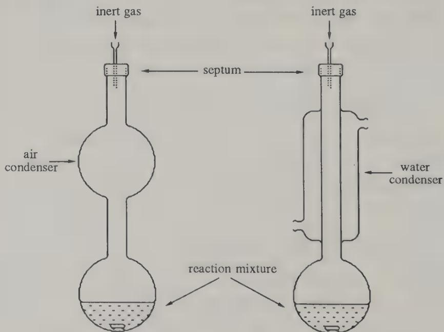
Figure 10.4 Small scale air condenser and water condenser systems.
