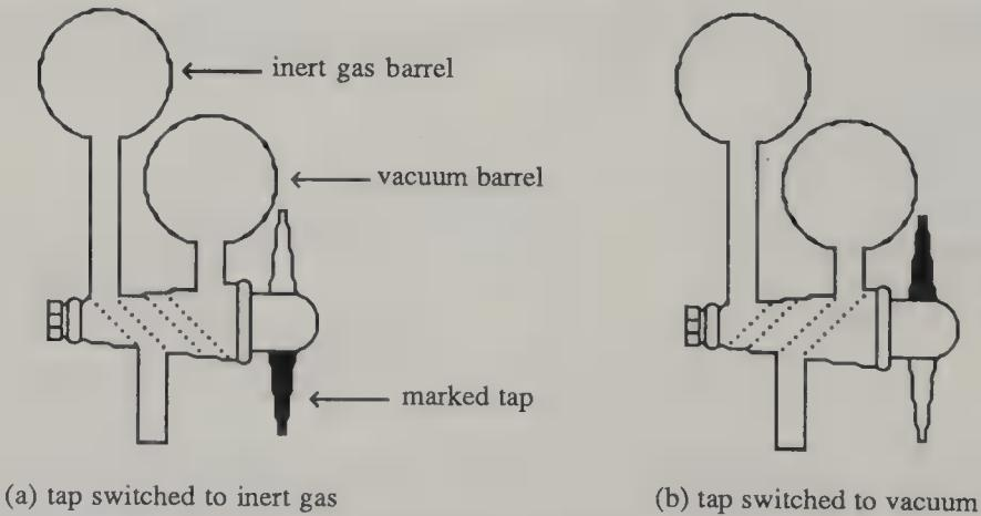
Figure 3.5 Cross section through a double oblique tap
