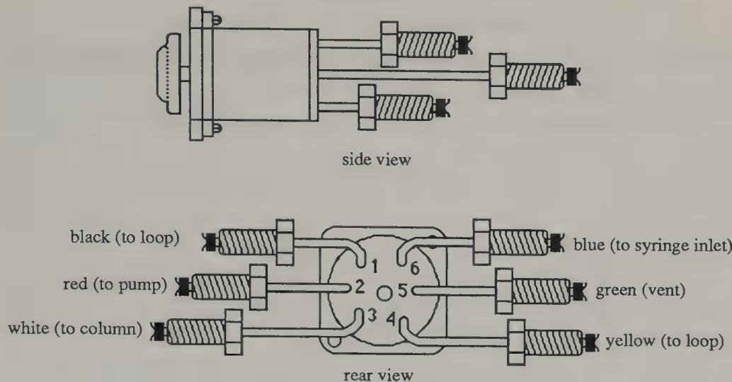
Figure 9.25 Rheodyne Type 50 mpc injection valve
