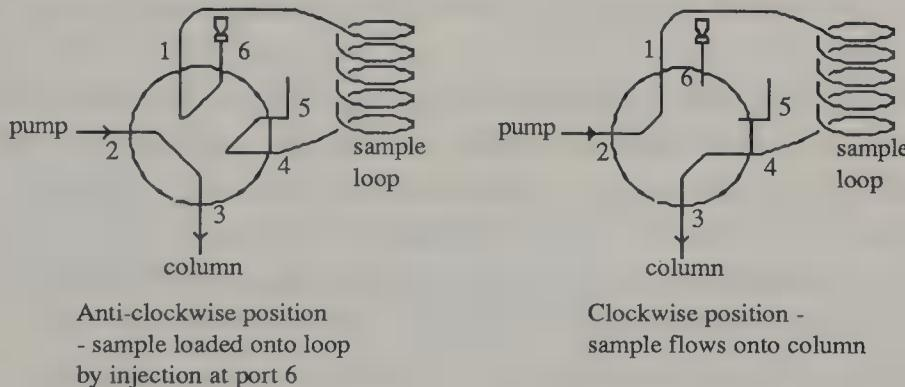
Figure 9.26 Flow through mpc injection valve
