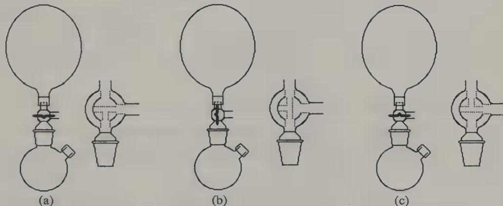
Figure 14.2 Small scale hydrogenation using a balloon
