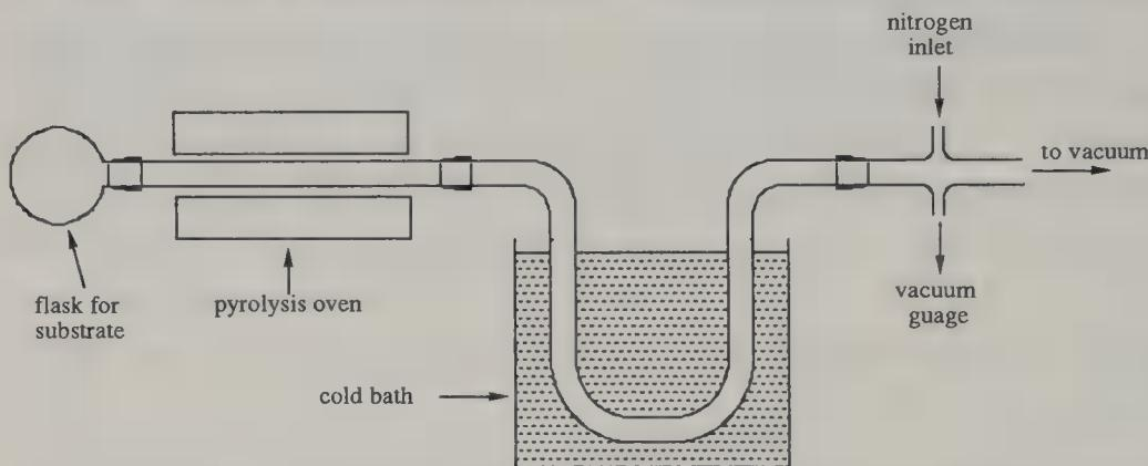
**Figure 14.4** Schematic representation of an apparatus for FVP
