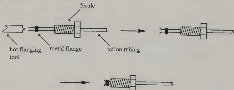
Figure 9.23 Fitting a ferule to 3mm teflon tubing
