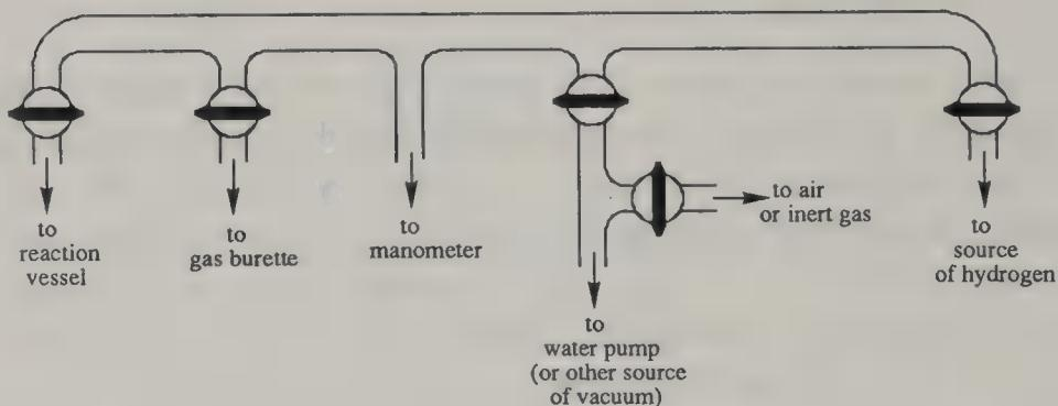
Figure 14.1 Schematic diagram of an atmospheric hydrogenator
