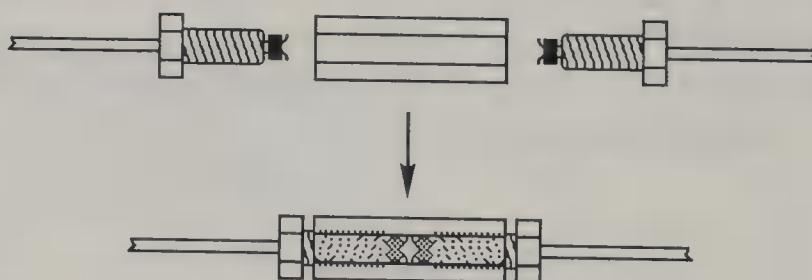
Figure 9.24 Connecting 3mm tubing using a threaded sleeve
