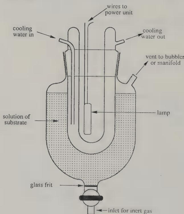
**Figure 14.3** Photochemical reactor
