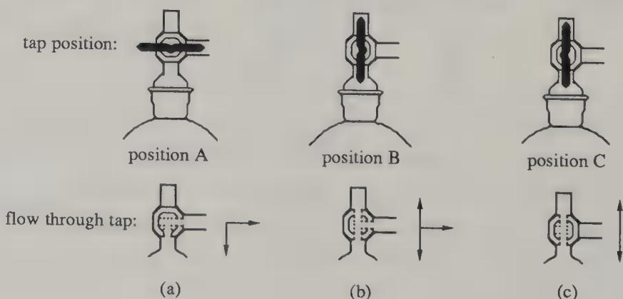
Figure 8.2 Flow through a 3-way tap relative to tap position.
