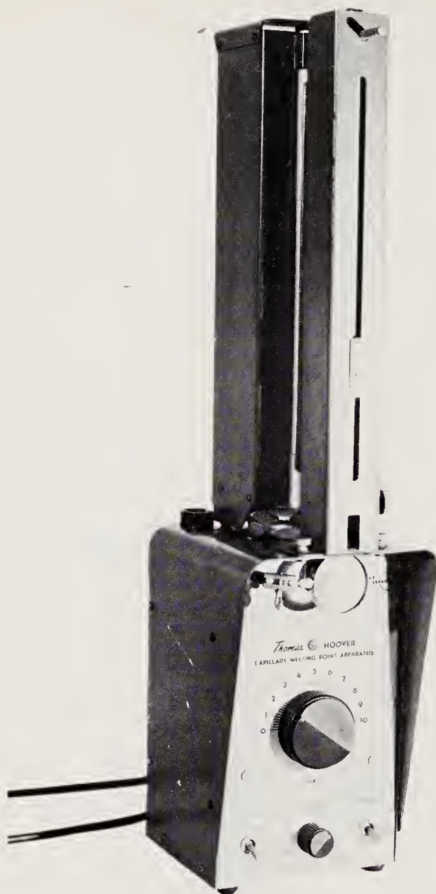
Figure 1.4 Thomas-Hoover melting-point determination device.
