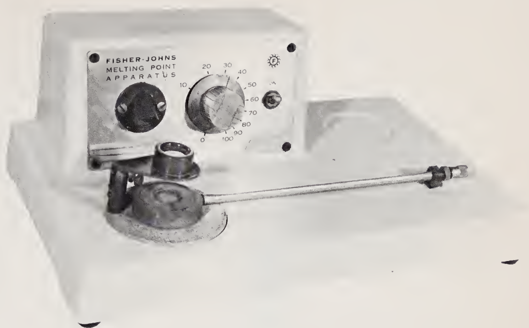
Figure 1.5 Fisher-Johns melting-point apparatus, an example of the so-called hot-stage melting-point apparatus. See text for additional discussion.
