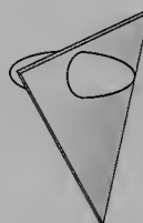
Fig. 2.17 Triangular spin vane for magnetic stirring in conical reaction vials.
