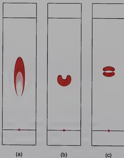
Fig. 3.69 Commonly encountered strangely shaped TLC spots from pure materials: (a) substance contains strongly acidic or basic groups; (b) adsorbant surface disturbed on application; (c) compound applied as solution in very polar solvent.
