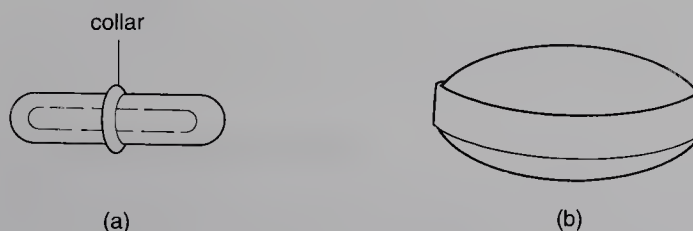
Fig. 2.13 Useful shapes of Teflon®-coated bar magnet.
