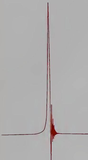
Fig. 5.27 Typical line shape obtained on a CW spectrometer. The 'wiggles' following the line are absent from spectra obtained in FT mode.
