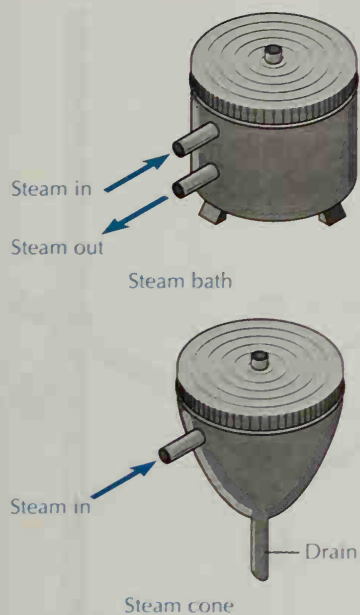
FIGURE 3.4 Devices for heating liquids below 100°C.
