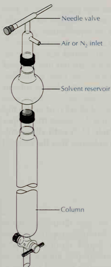
FIGURE 12.6 Apparatus for flash chromatography.
