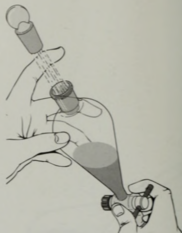
FIGURE 4.5 Failure to vent the separatory funnel when washing with sodium carbonate or bicarbonate solution can cause the stopper to blow out.
