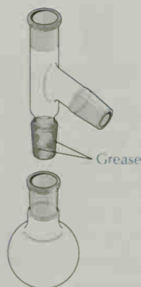
FIGURE 2.3 Assembling standard taper joint on macroscale glassware. Apply two thin strips of grease that run the entire length of the inner joint and are about 180° apart. Insert the inner joint into the outer joint and rotate one of the pieces. The joint should rotate easily and show a clear band of grease on its entire surface.
