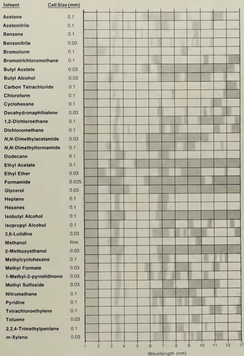
Figure 5.10 Chart of solvents for use in the infrared region. The unshaded areas represent useful regions in which transmittance of the pure solvents is > 60%. (Re-produced by courtesy of Eastman Kodak Company, Rochester, N.Y.)
