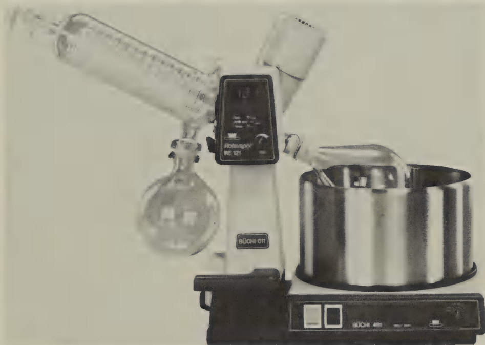
Figure 1.15 A Büchi rotary evaporator. (Reproduced by courtesy of Büchi/Brinkman Instruments, Inc., Westbury, N.Y.)
