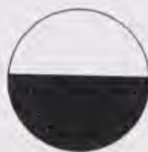
Figure 10-3 Visual Field for Properly Adjusted Refractometer
