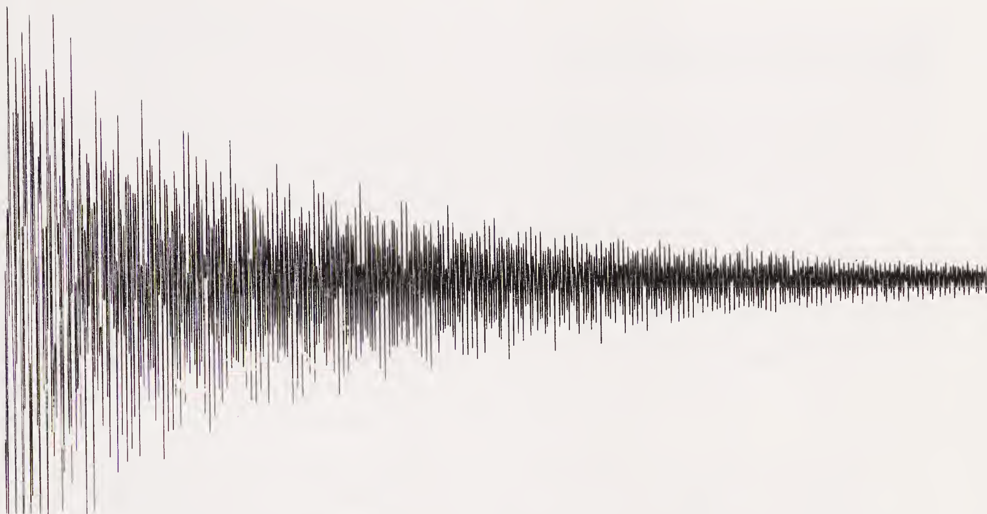
Fig. 6.3. (b) Free induction decay signal of benzyl acetate.
