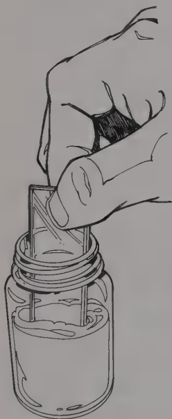
FIGURE 16.6 Preparation of TLC plates by dipping. The two microscope slides are grasped at one end, dipped into the silica gel slurry, removed and separated, and dried and activated by heating.
