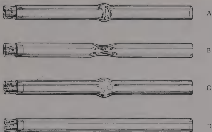
FIGURE 60.6 Making a straight seal.
