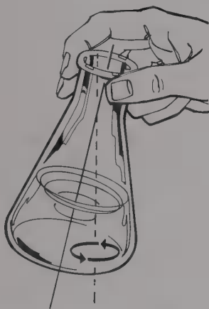
FIGURE 1.18 Swirling a liquid in a flask. The bottom of the flask is given a circular motion, the top remains stationary.
