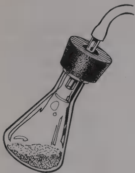
FIGURE 4.8 Drying a solid by reduced air pressure.
