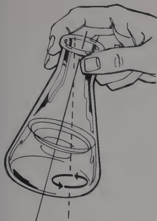
FIGURE 4.3 Swirling of a solution.
