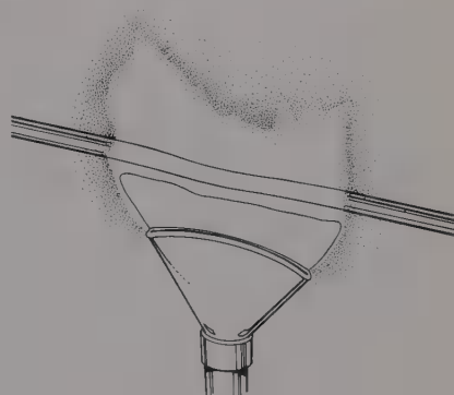
FIGURE 60.3 Heating glass tubing prior to bending. The wing top produces a broad flame that heats enough of the tubing to allow a good bend to be made. The tubing is held about 7 mm above the inner blue flame.
