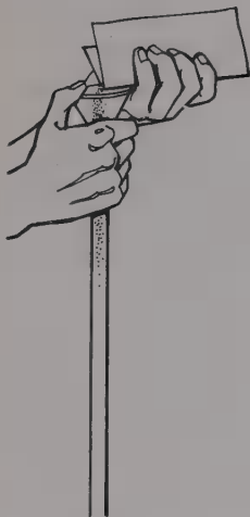
FIGURE 16.3 Technique useful when filling a chromatographic tube with alumina.
