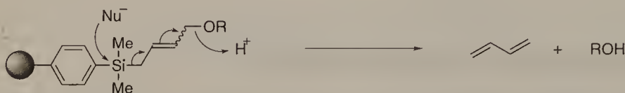
Scheme 3. Proposed mechanism for the protodesilylation of the polymer-bound metathesis products formed from allyl ethers or esters
