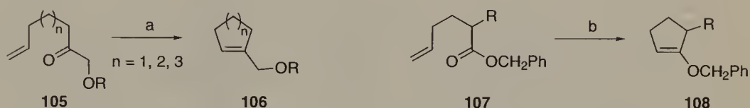
Scheme 15. Olefin metathesis-carbonyl olefination. (a) Mo(=CHCMe 2 Ph){N[2,6-( i -Pr) 2 C 6 H 3 ]}[OCMe(CF 3 ) 2 ] 2 (1), 84–86%; (b) W(=CHCMe 3 ){N[2,6-( i -Pr) 2 C 6 H 3 ]}[OCMe(CF 3 ) 2 ] (109) (Grubbs et al.) [31]
