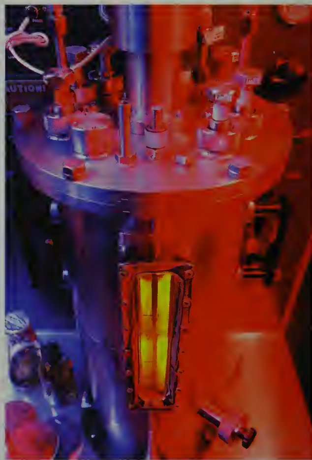
Figure 3.4 Modern fermentation vessel used for the production of penicillins.
