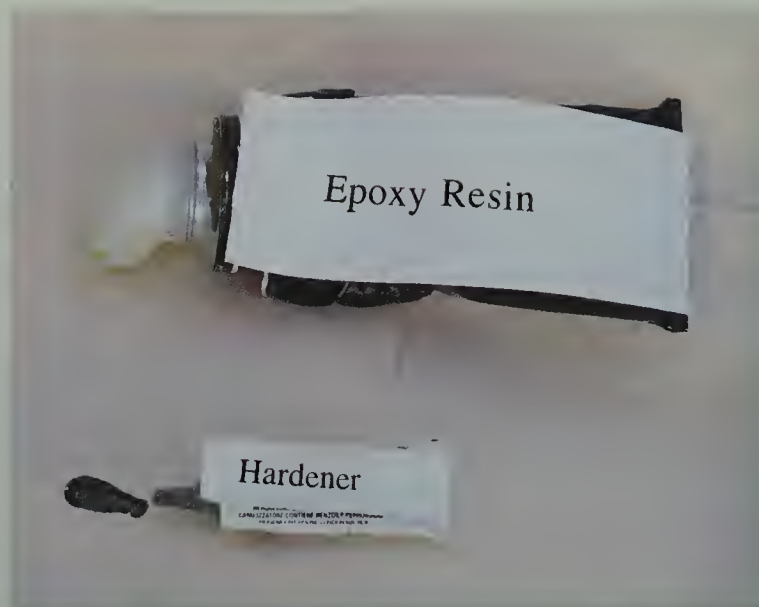
Figure 1.5 The two components of a typical epoxy resin glue.
