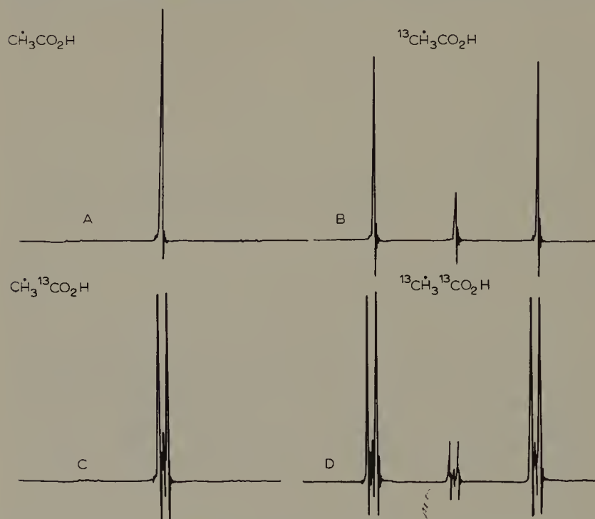
Fig. 3 (A) Natural abundance ^1\text{H} -n.m.r. spectrum of the methyl group protons of acetic acid. (B) ^1\text{H} -n.m.r. spectrum of the methyl group protons of acetic acid with the methyl carbon enriched to 90% with ^{13}\text{C} . (C) ^1\text{H} -n.m.r. spectrum of the methyl group protons of acetic acid with the carboxyl carbon enriched to 90% with ^{13}\text{C} . (D) ^1\text{H} -n.m.r. spectrum of the methyl group protons of acetic acid with 90% ^{13}\text{C} enrichment at both carbons.
