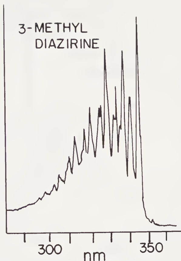
FIGURE 2. The UV absorption spectrum of MD. The band extends from 294 to 350 nm; it consists of many sharp lines with the maximum at 341 nm, where the absorption coefficient is 470 \text{ dm}^3/\text{mol}/\text{cm} . (From Frey, H. M., in Advances in Photochemistry , Vol. 4, Noyes, W. A., Jr., Hammond, G. S., and Pitts, J. N., Eds., John Wiley & Sons, New York, 1966, 225. With permission.)
