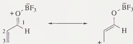
Figure 13 Enol resonance structure of BF_3 /enal complexes
