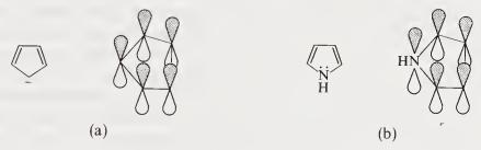
Fig. 2.6 Representations of the structure of the cyclopentadienyl anion (a) and of pyrrole (b).
