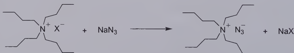
Scheme 2.7 Synthesis for the production of TBAA
