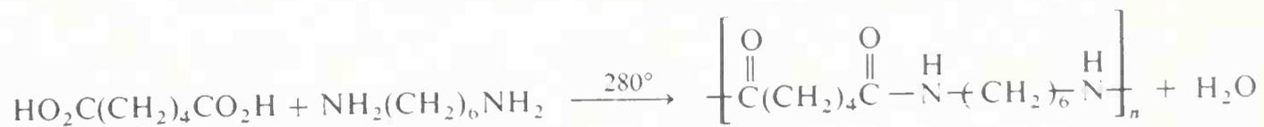
The polymer can be converted into fibers by extruding it above its melting point through spinnerettes, then cooling and drawing the resulting filaments. It is also used to make molded articles. Nylon (66) is exceptionally strong and abrasion resistant.
